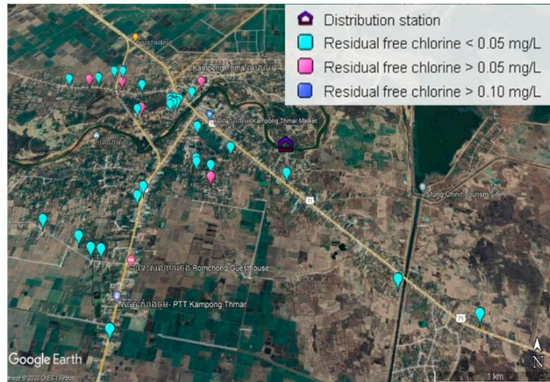
Figure 2. Field monitoring of residual chlorine in NN.
