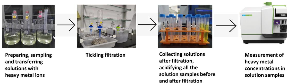
**Figure 2.** Procedural concept of the tickling filtration experiment with ERC/nano-ERC made with recycled aggregates and copper oxide nanoparticles to remove heavy metals from a simulated wastewater effluent.
