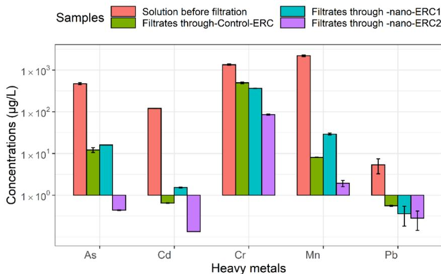
**Figure 3.** Heavy metal (HM) concentrations before and after filtration through control-ERC/ nano-ERC made with recycled aggregates and copper oxide nanoparticles (concentrations in the y axis were log-transformed in order to make the difference between treatments more visible).
