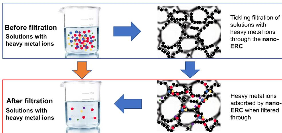
**Figure 5.** The procedural mechanisms of nano-ERC made with recycled aggregates and copper oxide nanoparticles adsorbing heavy metals (colorful dots in the solution are different heavy metal ions; black dots in the pore of concrete are nCuO).
