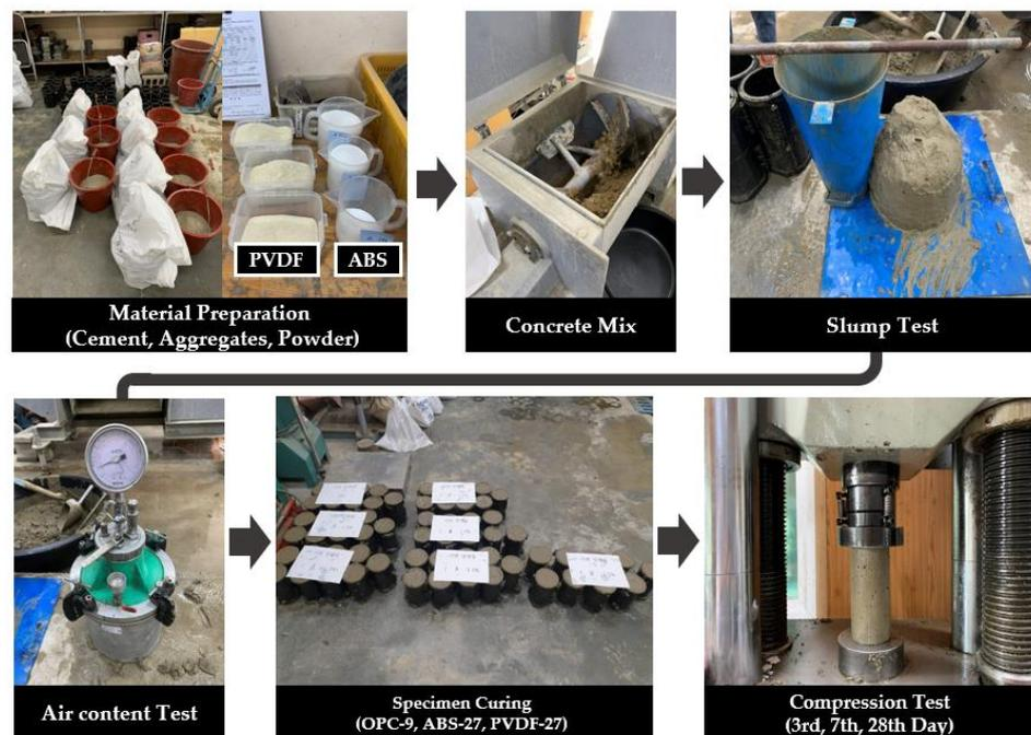
**Figure 3.** Testing process for ABS/PVDF concrete.
