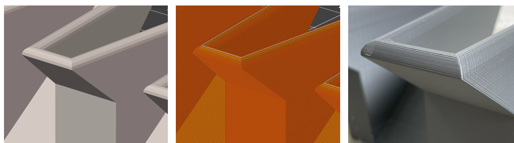
Figure 4. From digital data to final model, left: STL model, middle: sliced layer model, right: final print.
