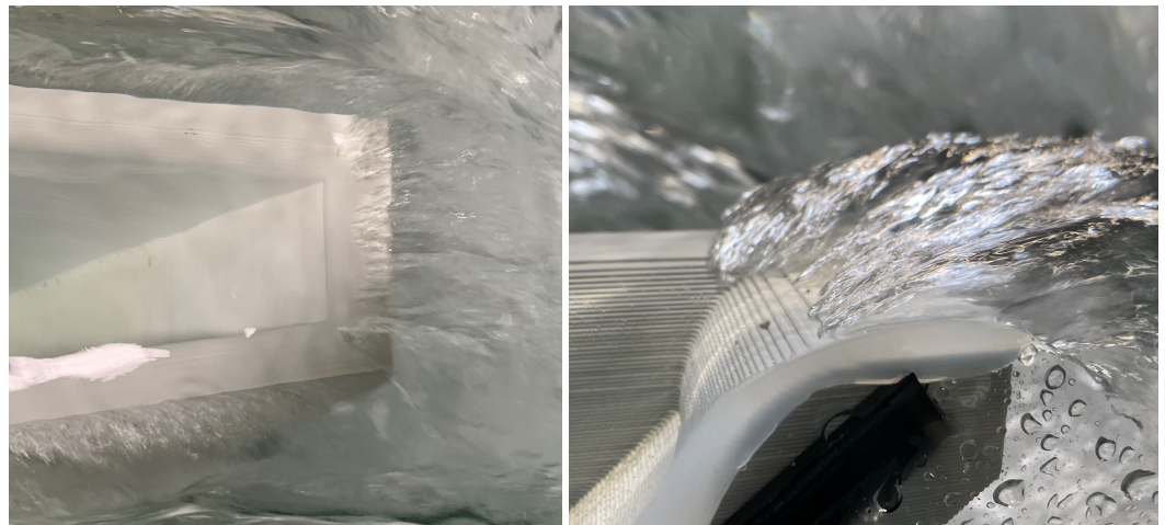
Figure 9. Detail of nappe separation induced by surface roughness, TPKW P40 , left: top view, right: side view, flow direction from left to right.
