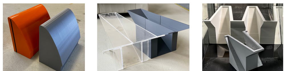
Figure 2. Investigated weir geometries, left: regular linear weirs, middle: rectangular piano key weirs, right: trapezoidal piano key weirs.
