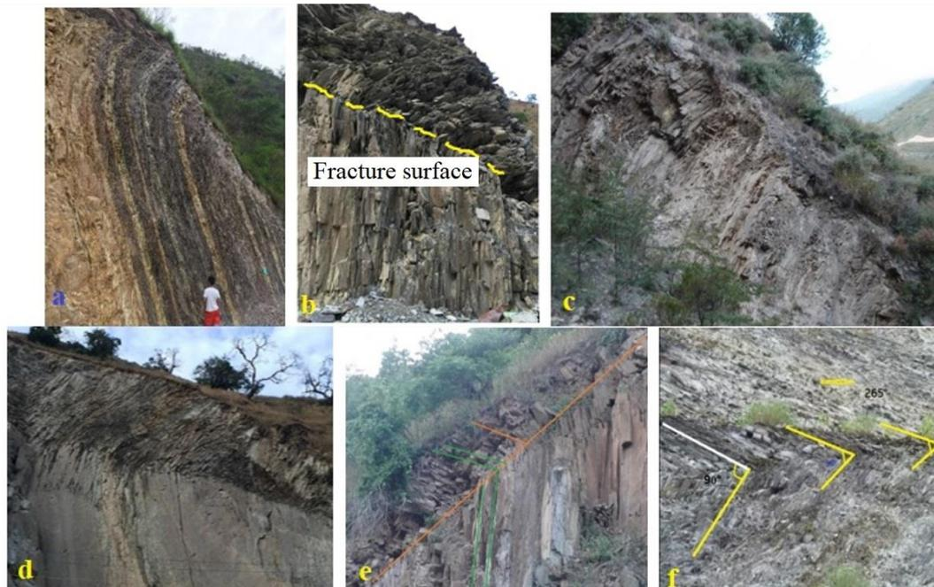
**Figure 4.** (a) Metasandstone toppling deformation at Qingcaiping on the left bank. (b) toppling shallow broken in metasandstone. (c) toppling broken face in consequent slope. (d) toppling broken face in reverse slope of metasandstone. (e) toppling bending in slate. (f) slate toppling deformation body at the crossing road downstream of Biaocun town on the right bank.
