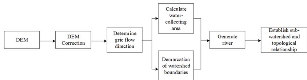
**Figure 2.** Schematic diagram of sub-watershed division process and establishment of confluence relationships.
