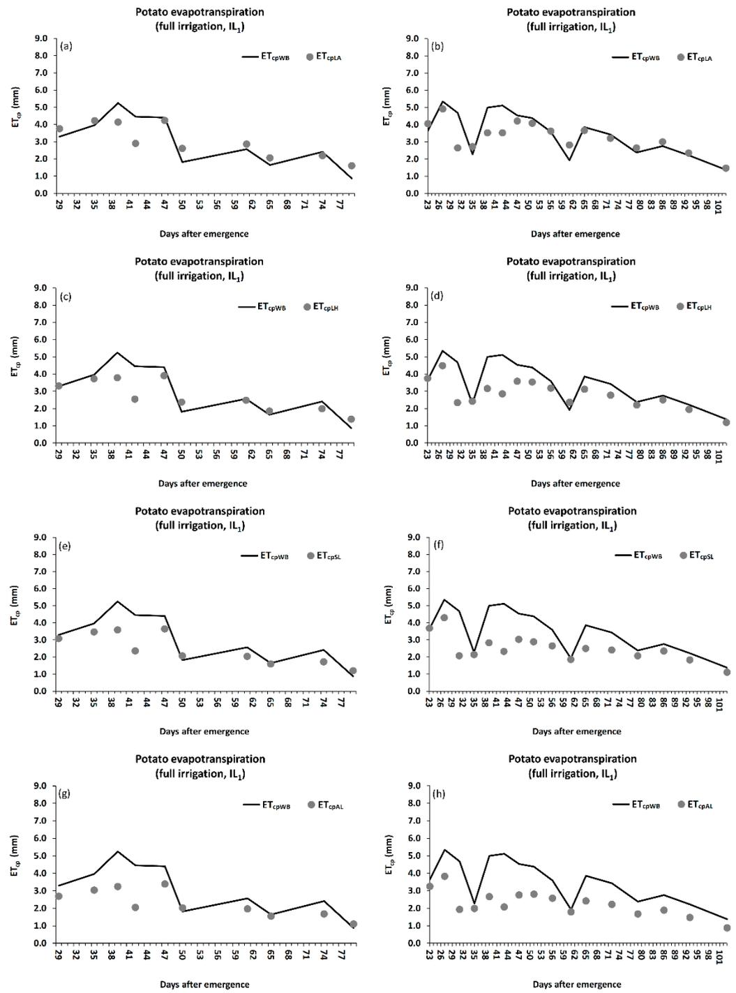
**Figure 10.** Comparison of daily average  $ET_{cp}$  by soil water balance method and PM method with different canopy resistance approaches on a full irrigation condition (IL<sub>1</sub>) for 2018/2019 (a,c,e,g) and 2019/2020 seasons (b,d,f,h).
