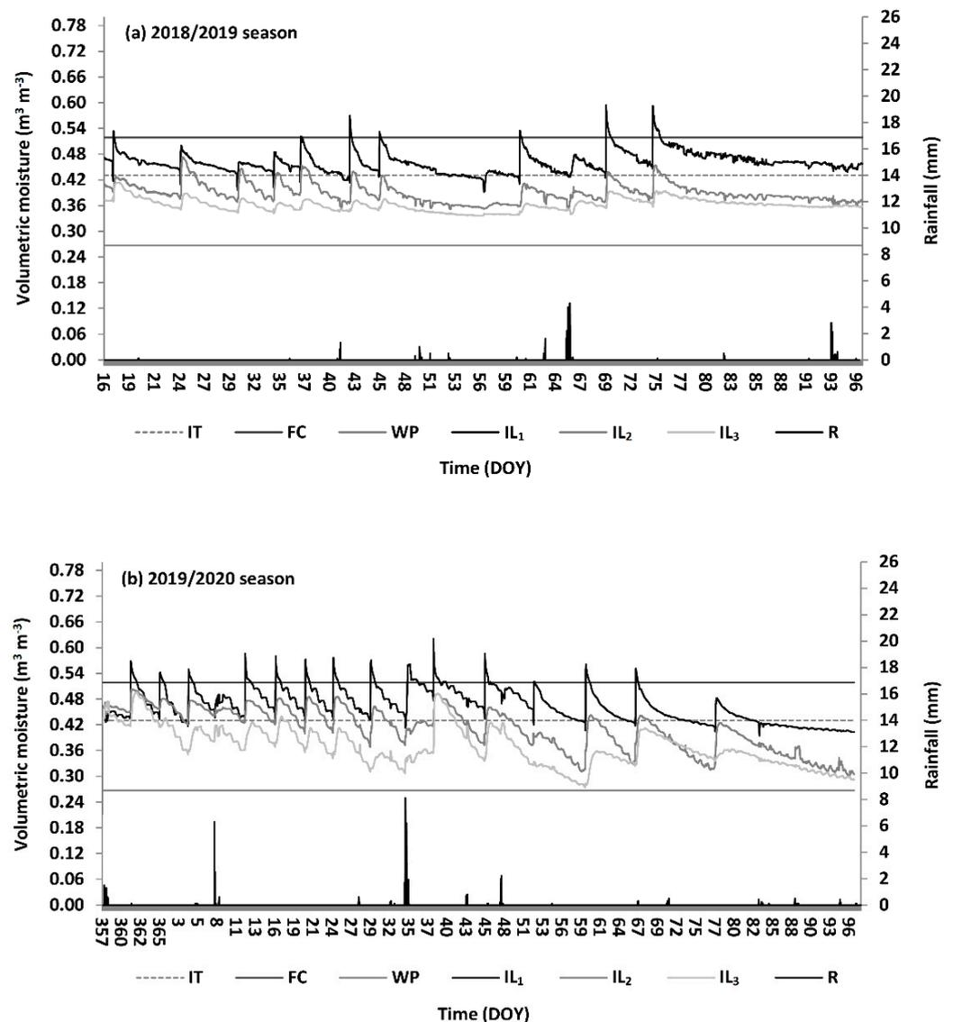
**Figure 3.** Variation of volumetric soil water content and rainfall measured values for the two evaluated seasons 2018/2019 (a) and 2019/2020 (b). The irrigation level (IL) was  $IL_1$ : Full irrigation,  $IL_2$ : 75% of  $IL_1$ , and  $IL_3$ : 60% of  $IL_1$ . IT, R, FC, and WP are irrigation threshold, rainfall, and soil water content at field capacity and permanent wilting point.
