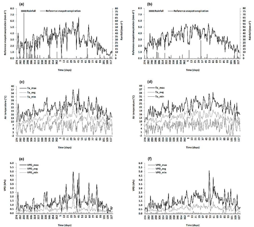
**Figure 2.** Daily variation of meteorological data registered by an automatic weather station (AWS) located close to study site for the 2018/2019 (a,c,e) and 2019/2020 (b,d,f) seasons.  $T_a$  is the air temperature, and VPD is the vapour pressure deficit. The abbreviation max, avg and min are the measured variables' maximum, average, and minimum expression.
