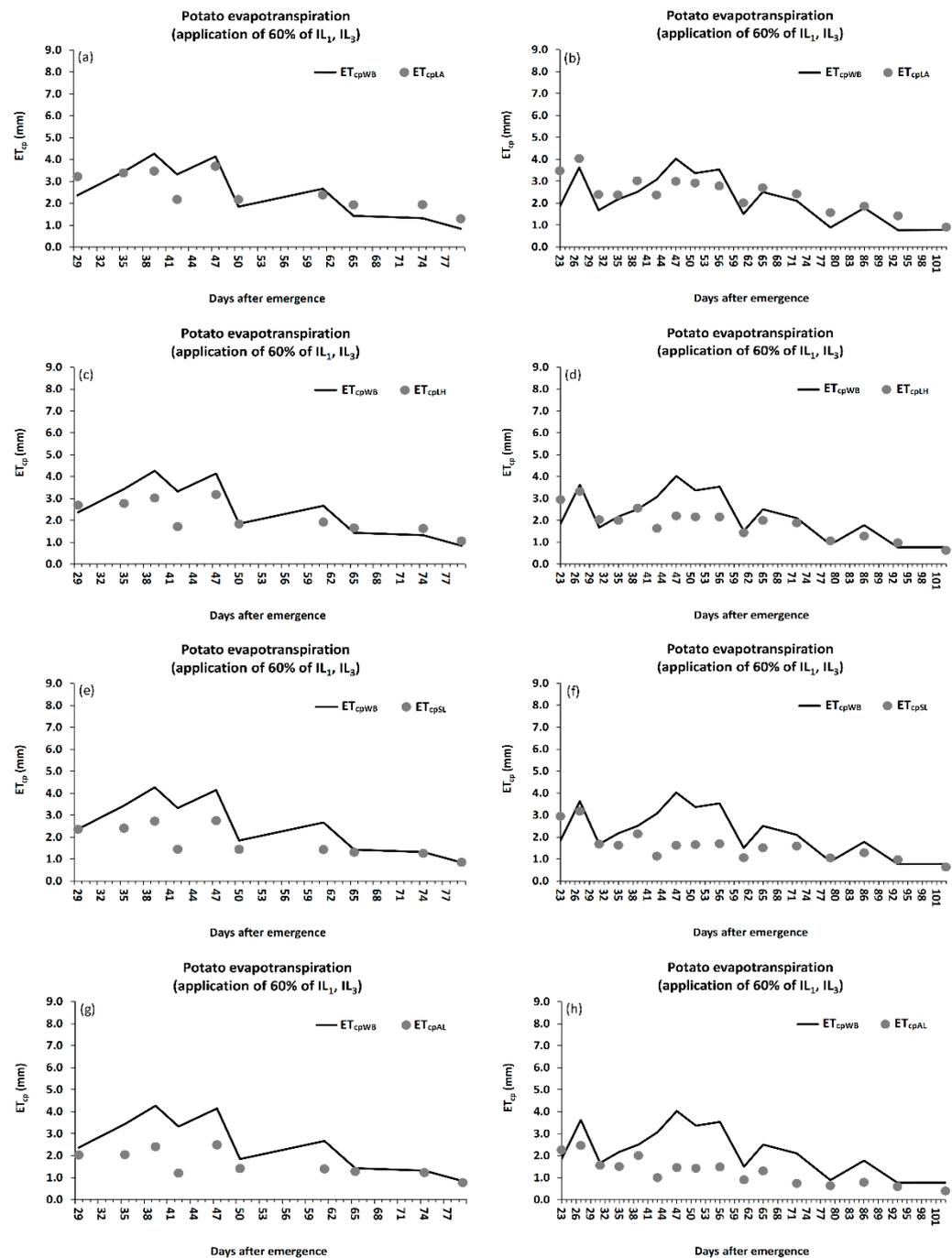
**Figure 12.** Comparison of daily average  $ET_{cp}$  by soil water balance method and PM method with different canopy resistance approaches on an application of 60% of  $IL_1$  ( $IL_3$ ) for 2018/2019 (a,c,e,g) and 2019/2020 seasons (b,d,f,h).
