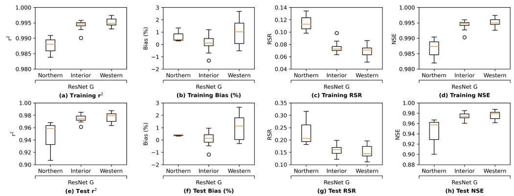
**Figure A16.** Box and whisker plots of four types of metrics consisting of  $r^2$ , percent bias, RSR, and NSE on stations belonging to the northern, interior, and western Delta groups during the training (panels (a–d)) and test (panels (e–h)) phases of the grouped (G) ResNet model.
