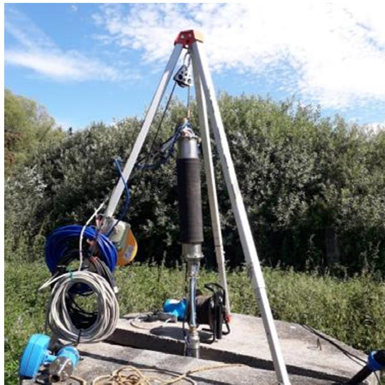
**Figure 11.** The INV-FLOW apparatus during installation in the measured extraction well HJ-3 at the pilot site.
