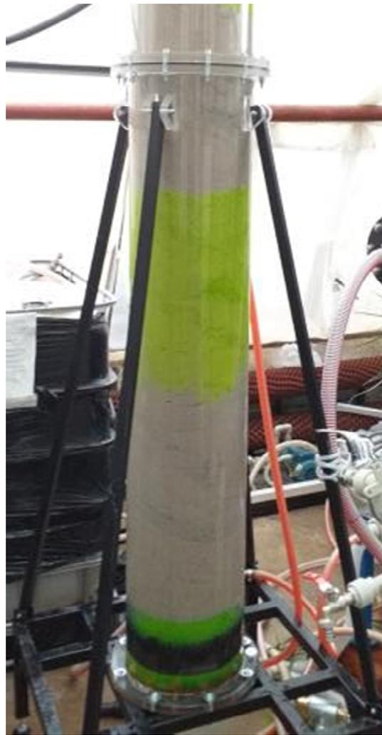
**Figure 7.** The laboratory tracer test carried out in Scenario C visually indicated the measuring area of the INV-FLOW apparatus.
