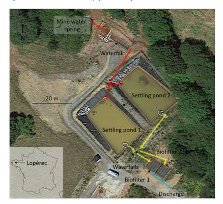
Figure 1. Lopérec mine drainage passive treatment system.
