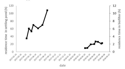
**Figure 2.** Evolution of hydraulic residence time (HRT) in the settling pond and in the biofilter in 2017 and in 2018. The values for the settling pond and the biofilter are directly proportional (factor of 10) because they both depend on the same flow-rate and on fixed volumes. The left *Y*-axis gives the scale for the settling pond and the right *Y*-axis gives the scale for the biofilter.
