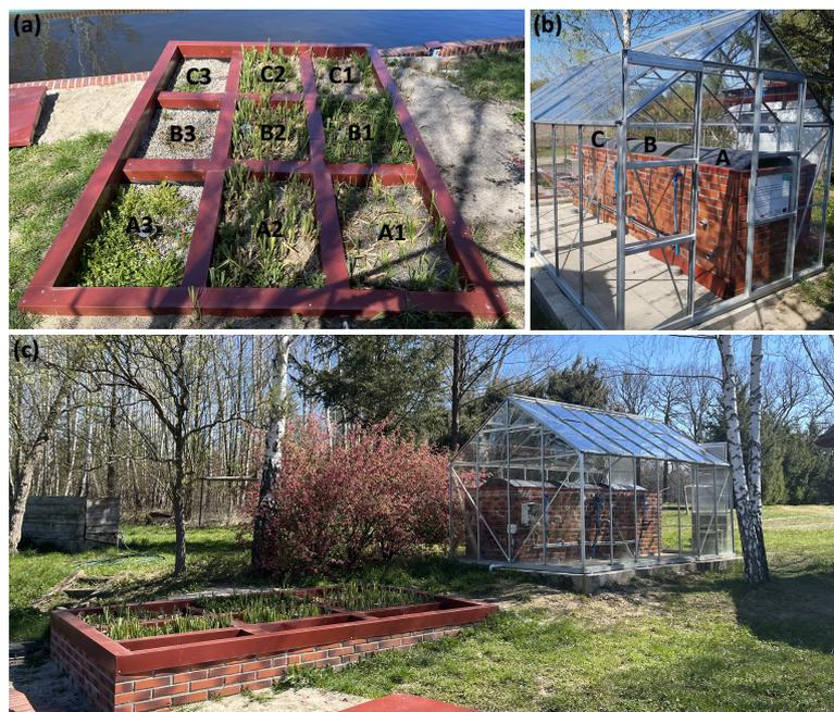
**Figure 2.** The pilot plant. A, B, C letters refer to the three different hydraulic loads (70, 100, and 130 l per day, respectively). (a) denitrification (1), phosphorus (2), and activated carbon (3) beds responsible for the water renewal, (b) compost beds responsible for the wastewater purification, (c) setting of the beds.
