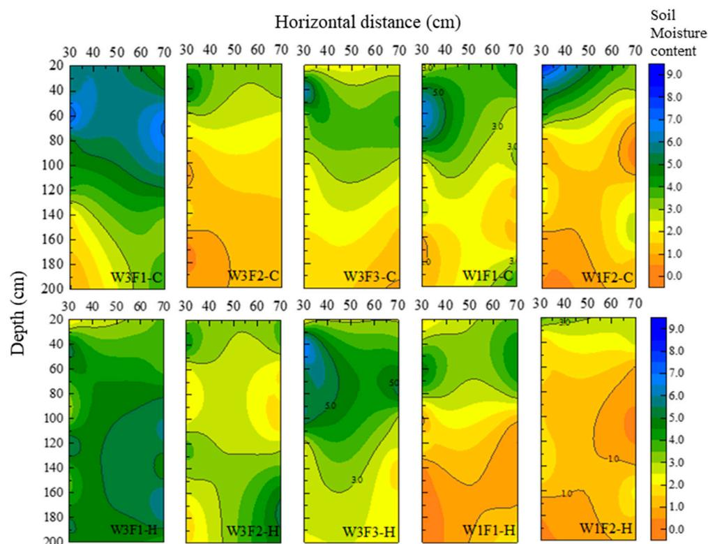
**Figure 4.** Spatial variation in soil moisture content under different irrigation periods. The soil moisture content in the low (W1), medium (W2), and high (W3) irrigation amounts. F means irrigation frequency with F1 = 10 d, F2 = 20 d, F3 = 40 d. C and H represent *C. mongolicum* and *H. ammodendron*, respectively.
