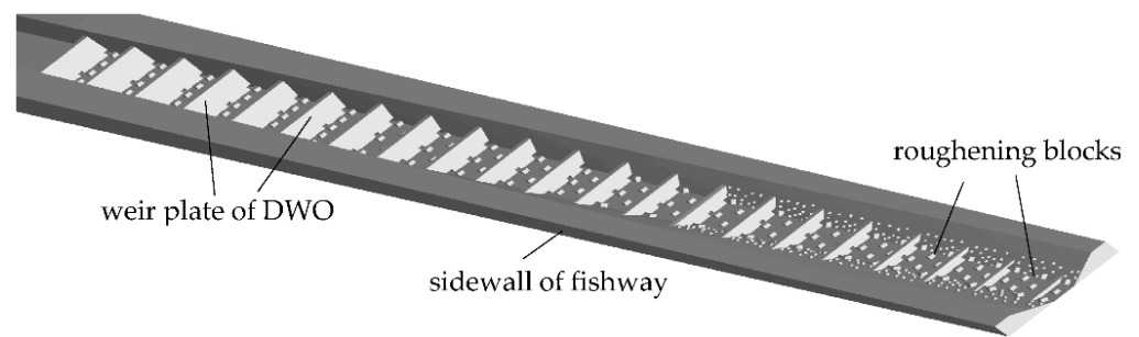
Figure 8. Three-dimensional numerical simulation model of the transition reach with the DWO. There are 21 multistage weirs and 61 orifices to maintain the flow discharge smoothly with double passages, and many bottom roughening blocks are set up to add roughness to the boundary so as to reduce the flow velocity, which is beneficial for resting fish.
