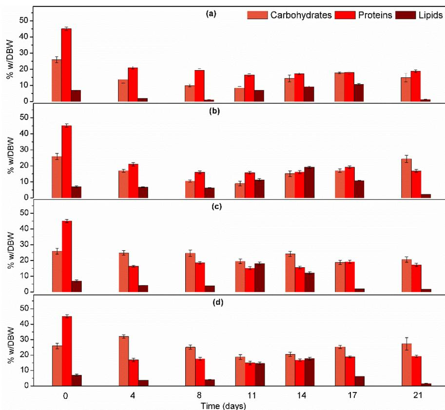
**Figure 3.** Carbohydrate, protein, and lipid contents in total biomass during *A. platensis* cultivation under continuous illumination in (a) untreated brewery wastewater, (b) brewery wastewater with 1 g/L NaCl, (c) brewery wastewater with 5 g/L NaHCO<sub>3</sub>, and (d) brewery wastewater with 1 g/L NaCl and 5 g/L NaHCO<sub>3</sub>. Data present mean values of duplicate experiments  $\pm$  standard deviations.
