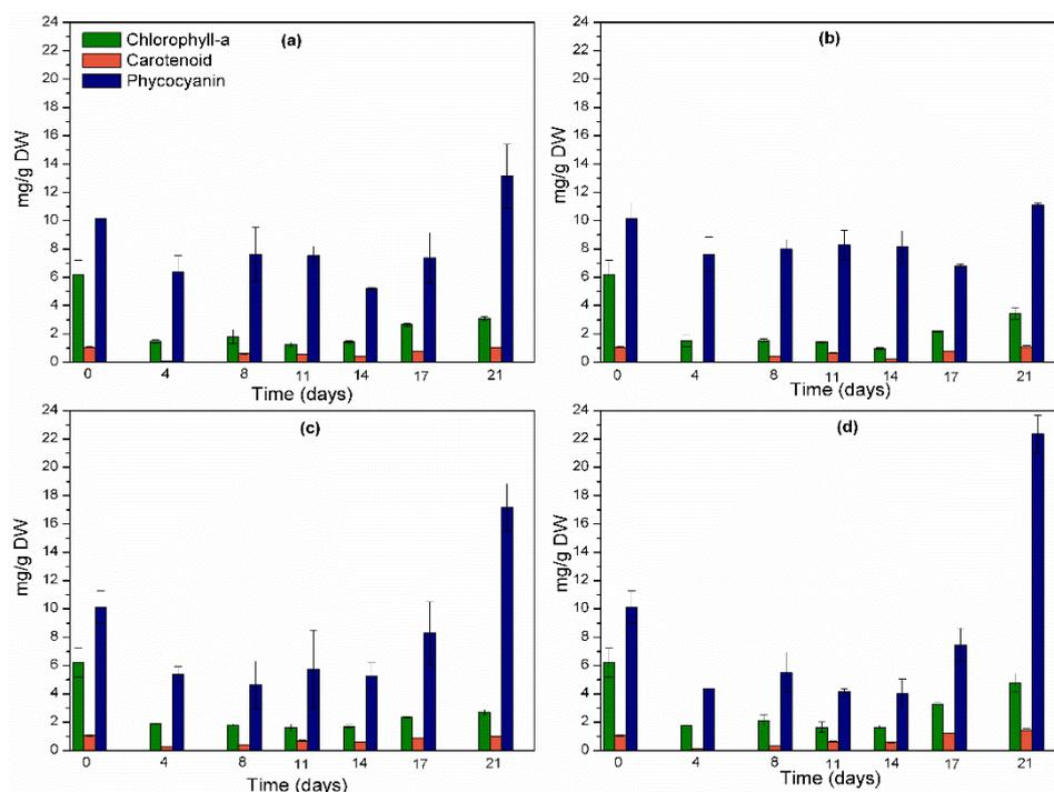
**Figure 2.** Pigments content into total biomass during *A. platensis* cultivation under continuous illumination in (a) untreated brewery wastewater, (b) brewery wastewater with 1 g/L NaCl, (c) brewery wastewater with 5 g/L  $\text{NaHCO}_3$ , and (d) brewery wastewater with 1 g/L NaCl and 5 g/L  $\text{NaHCO}_3$ . Data present mean values of duplicate experiments  $\pm$  standard deviations.
