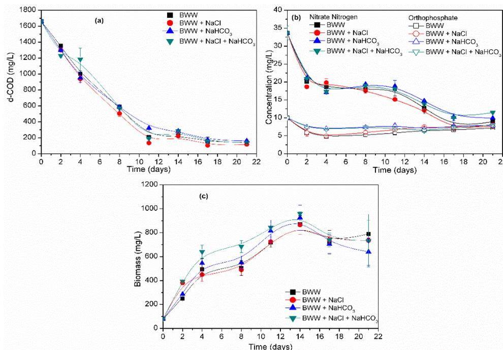
**Figure 1.** (a) d-COD consumption, (b)  $\text{NO}_3^-$ -N and  $\text{PO}_4^{3-}$ -P consumption, and (c) growth of total biomass during *A. platensis* cultivation under continuous illumination in four different brewery wastewater-based media. Data present mean values of duplicate experiments  $\pm$  standard deviations.
