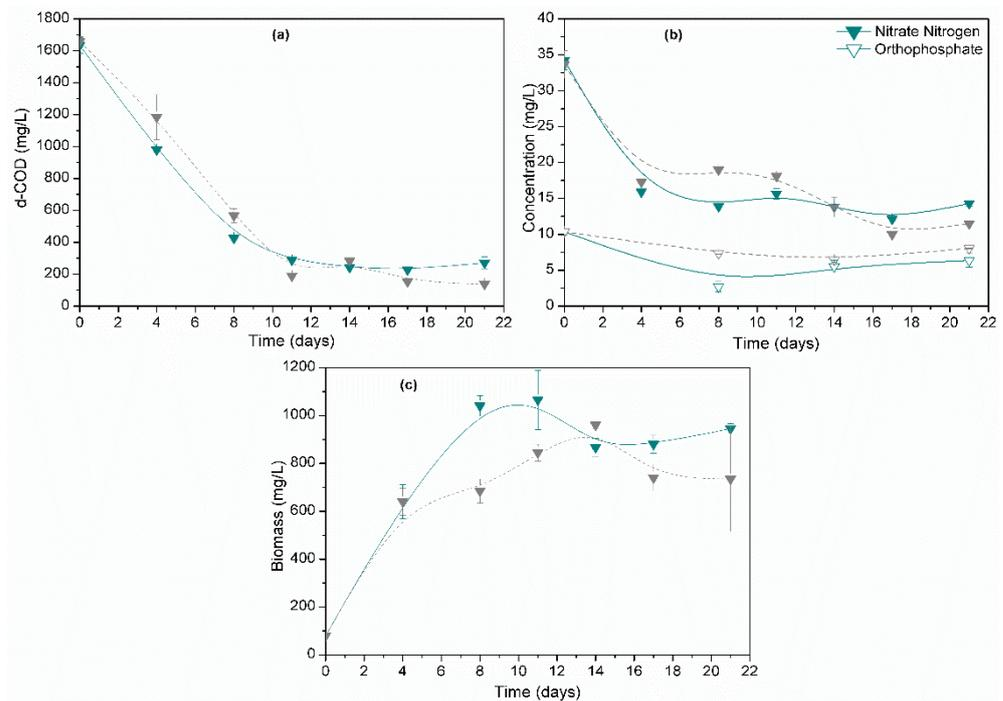
**Figure 4.** (a) d-COD consumption, (b)  $\text{NO}_3^-$ -N and  $\text{PO}_4^{3-}$ -P consumption, and (c) growth of total biomass applying photoperiod (16:8 h light:dark) during *A. platensis* cultivation in brewery wastewater with 1 g/L NaCl and 5 g/L  $\text{NaHCO}_3$ . Data present mean values of duplicate experiments  $\pm$  standard deviations. Grey symbols with dash lines represent the experiments conducted using the same brewery wastewater-based medium under continuous illumination.
