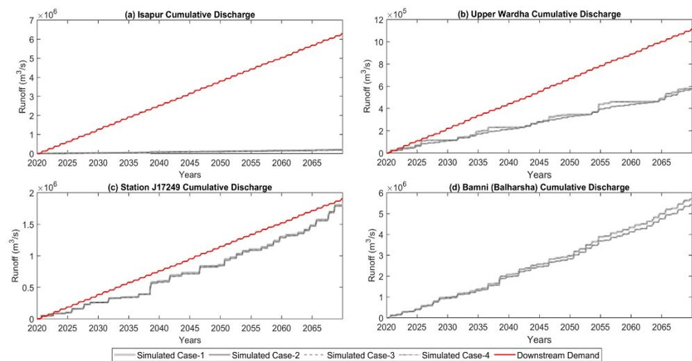
**Figure 14.** Cumulative hydrographs at four different stream gauge stations, namely, (a) Isapur Reservoir, (b) Upper Wardha Reservoir, (c) Station J17249 (immediate downstream station of Umarkhed Taluka), and (d) Bamni-Balharsha (outlet of the watershed), for RCP-8.5 climate change scenario and case 3 constraint combination of the optimization model.
