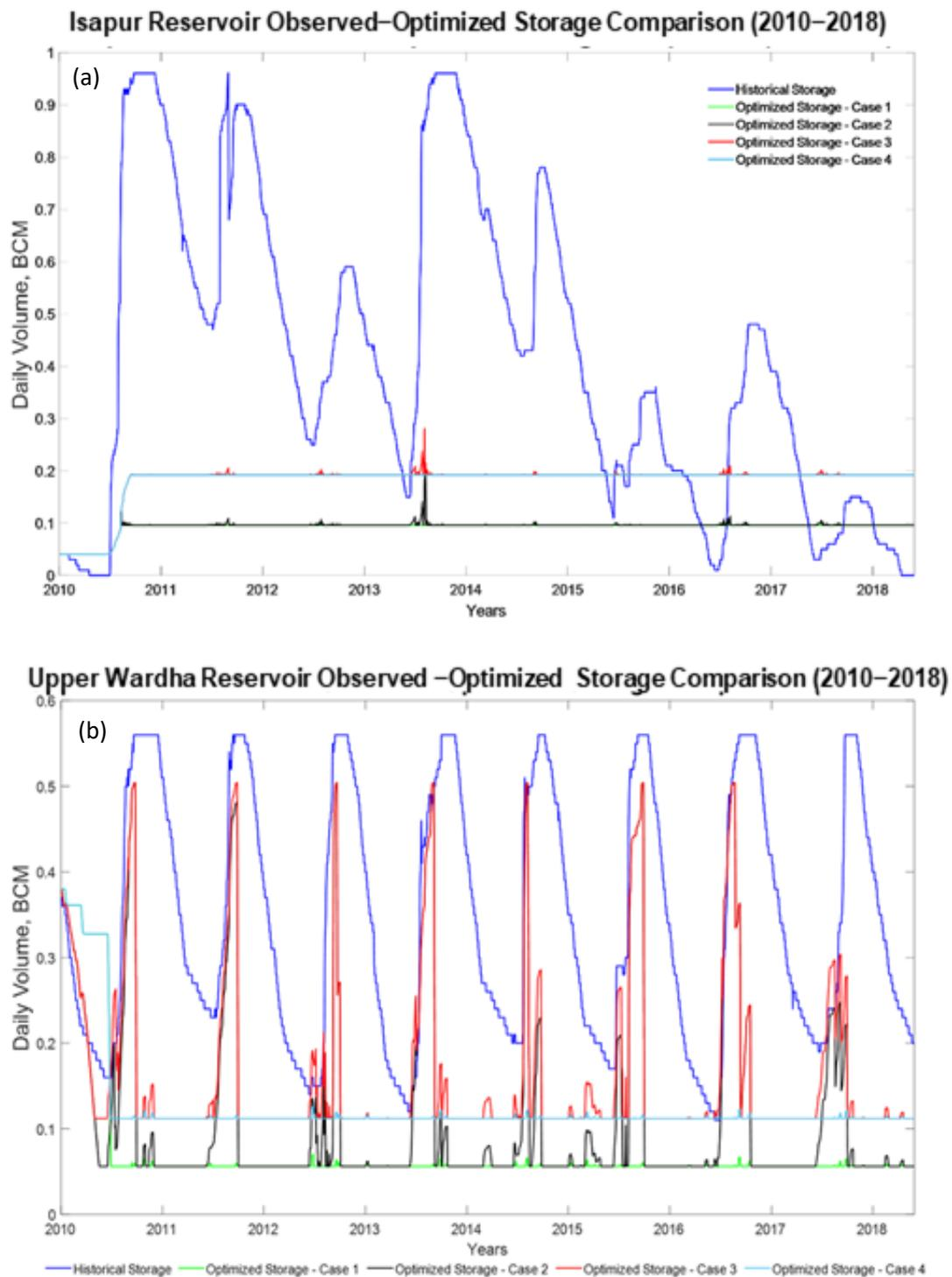
**Figure 9.** Comparison of observed–optimized storage for 2010 to 2018 of (a) the Isapur Reservoir, and (b) the Upper Wardha Reservoir.
