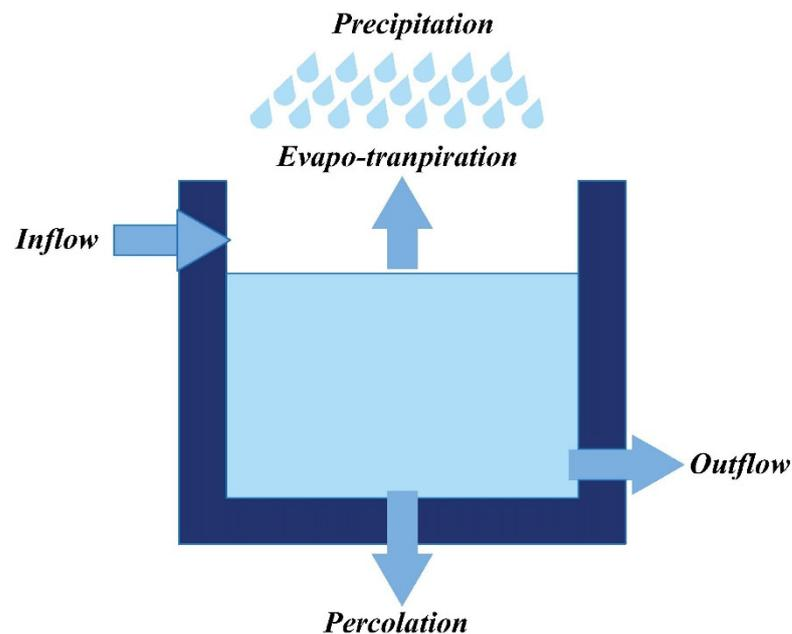
**Figure 7.** Illustration of mass balance of a reservoir.
