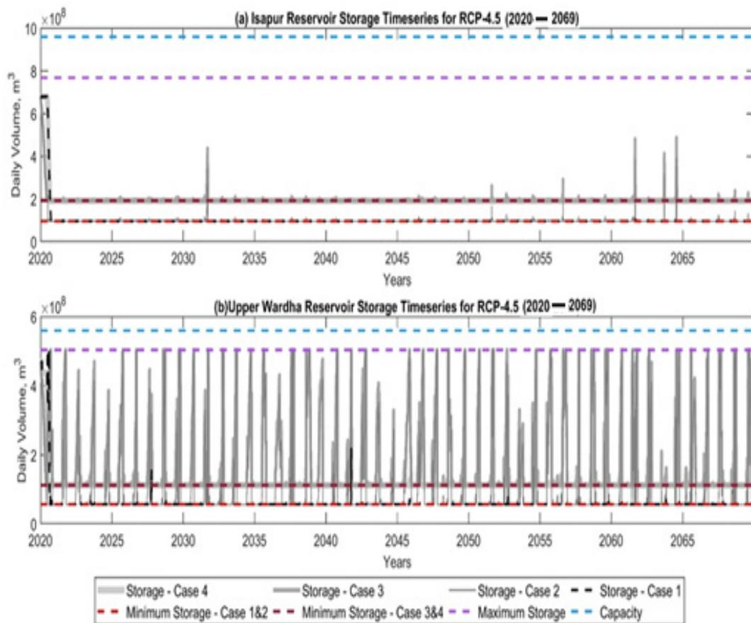
Figure 10. Optimized storage for RCP-4.5 scenario for 2020 to 2069 of (a) the Isapur Reservoir and (b) the Upper Wardha Reservoir.
