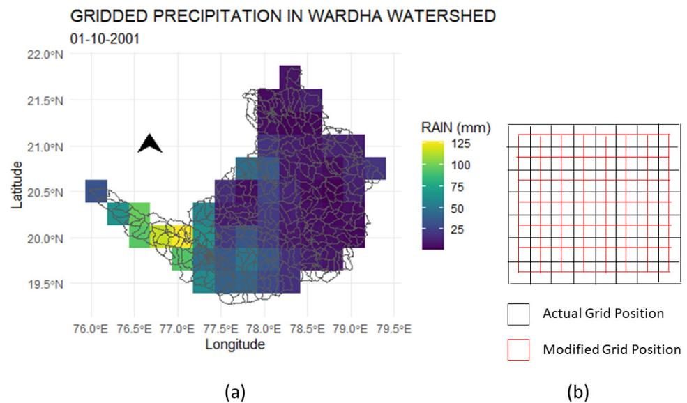
**Figure 3.** (a) Gridded precipitation pattern (sample date: 1 October 2001), and (b) grid coordinate transformation using interpolation for predicted rainfall time-series data. The black grids represent the predicted RCP rainfall grid location, and the red grids represent the modified grid position that overlaps with the historical rainfall grids.
