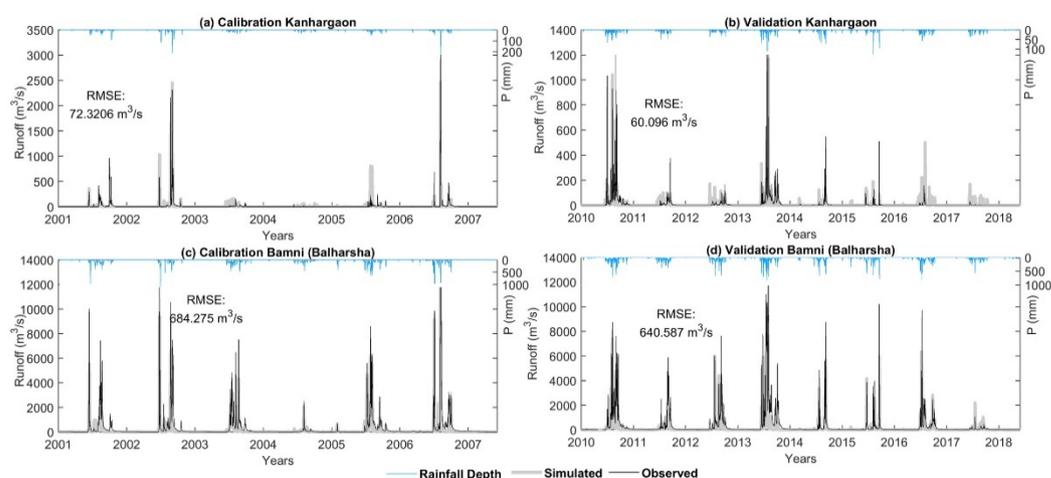
**Figure 6.** Comparison of calibrated–observed and validated–observed hydrographs at Kanhargaon and Bamni (Balharsha) stream gauge stations for observed rainfall hyetographs of their upstream sub-basins.
