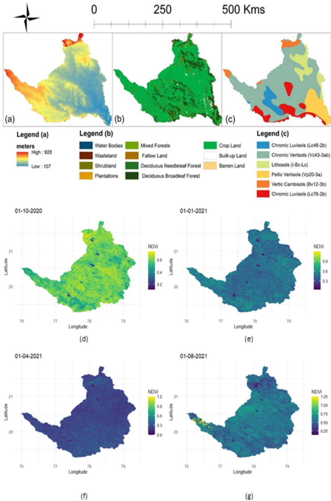
**Figure 2.** (a) Digital Elevation Model (DEM): the reddish border indicates the most upstream parts of the sub-basin where the blueish color defines the downstream part; (b) land use and land cover classification (2005): mostly agricultural land; (c) soil type map of the Wardha Watershed where a large portion of soil is Chromic Vertisols; (d–g) illustrate NDVI during different months of the water year 2021 ((d) October, (e) January, (f) April, and (g) July).
