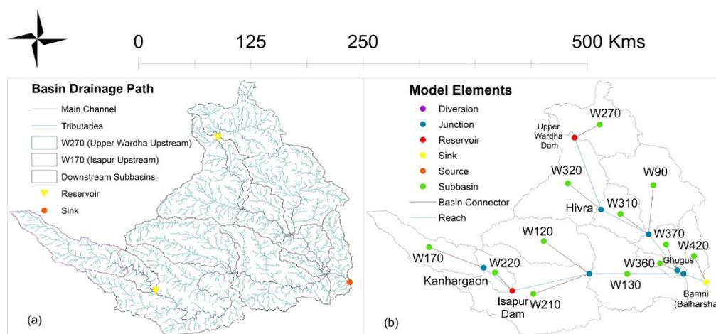
**Figure 5.** (a) Contributing area of the Wardha Watershed: the yellow triangles represent the location of the reservoirs, and the blue and magenta outlines indicate the upstream watersheds of the Upper Wardha and the Isapur dams, respectively; and (b) schematic representation of the basin model in HEC-HMS, where green, blue, and red circles represent the locations of the sub-basin centers, junctions, and dams, respectively.
