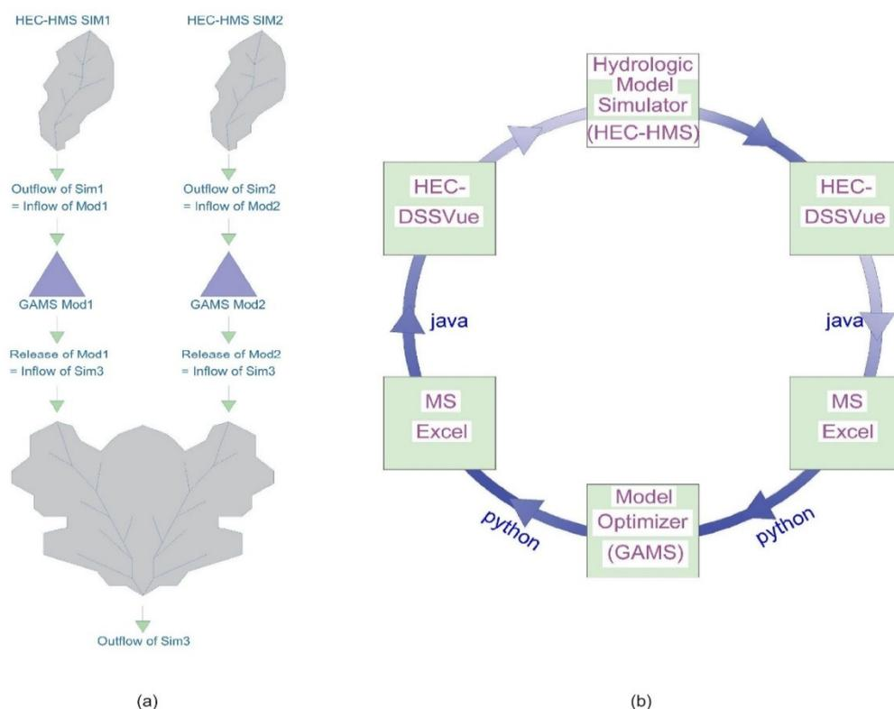
**Figure 8.** (a) Flow of the integrated hydrologic and optimization modeling method, and (b) stages of the optimization simulation model.
