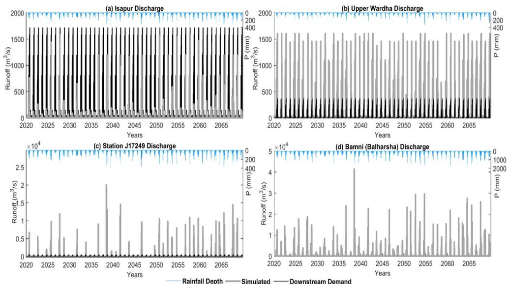
**Figure 13.** Hydrographs and rainfall hyetographs at four different stream gauge stations, namely, (a) Isapur Reservoir, (b) Upper Wardha Reservoir, (c) Station J17249 (downstream station of Umardhed Taluka), and (d) Bamni-Balharsha (outlet of the watershed), for RCP-8.5 climate change scenario and case 3 constraint combination of the optimization model.
