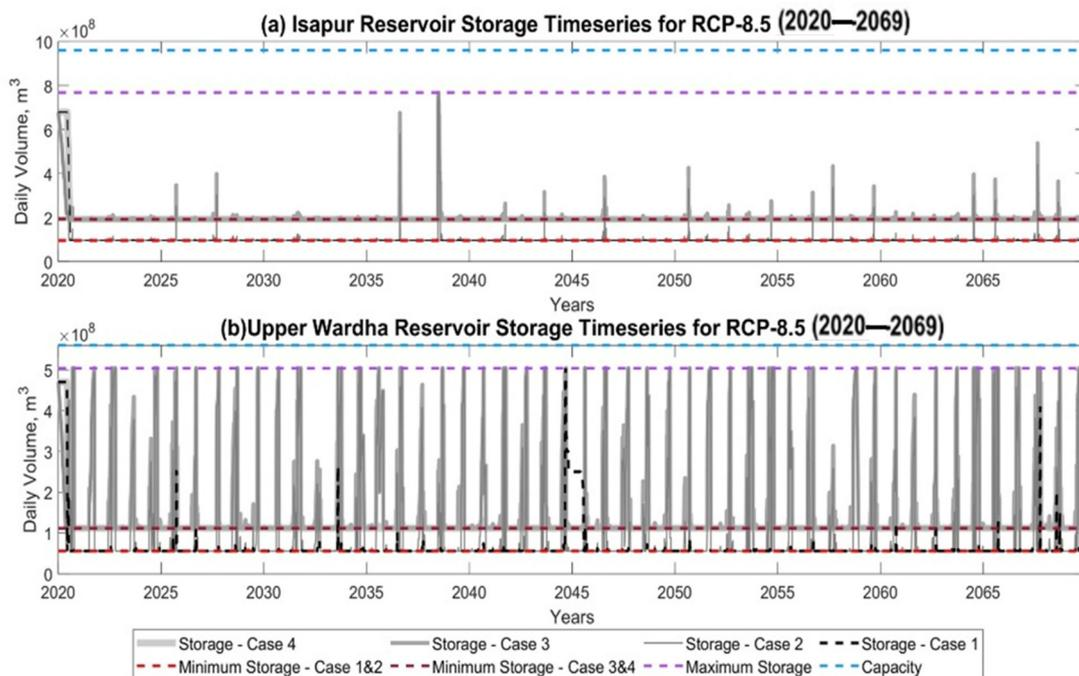
Figure 11. Optimized storage for RCP-8.5 scenario for 2020 to 2069 of (a) the Isapur Reservoir and (b) the Upper Wardha Reservoir.
