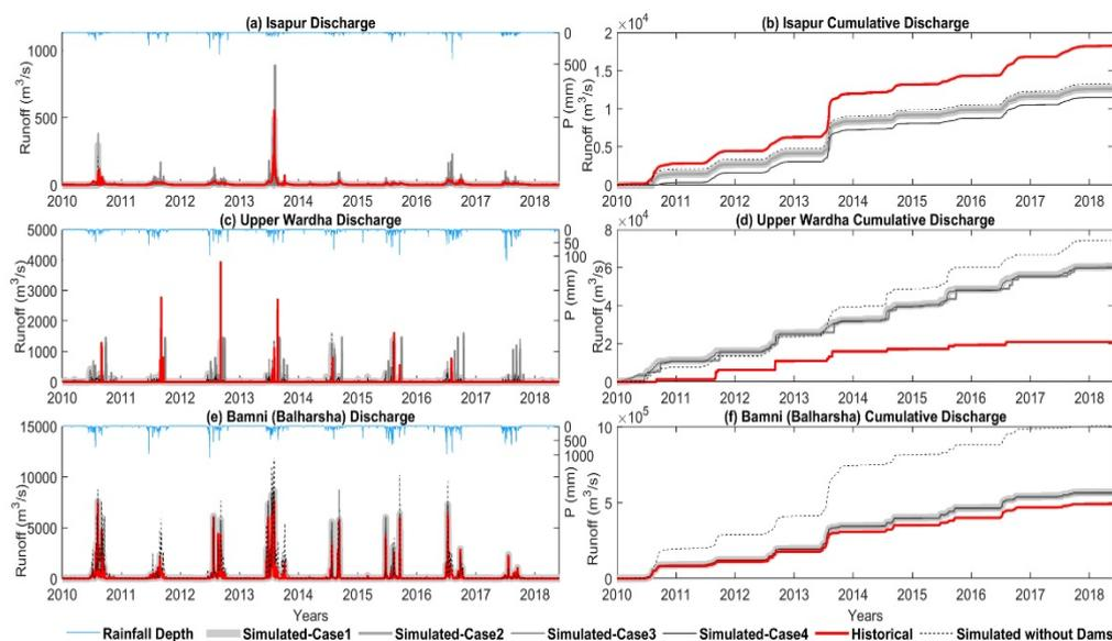
**Figure 12.** Comparison of observed and optimized discharge/cumulative discharge for different stations—(a) Isapur Reservoir releases, (b) Isapur Reservoir cumulative releases, (c) Upper Wardha Reservoir releases, (d) Upper Wardha Reservoir cumulative releases, (e) Bamni (Balharsha) discharge, and (f) Bamni (Balharsha) cumulative discharge.
