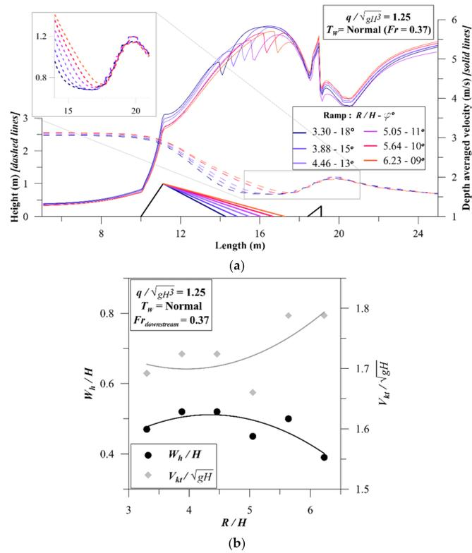
Figure 6. Effect of the ramp profile on the surf wave: (a) effect of the ramp steepness on wave profile and velocity distribution, (b) sensitivity of the surf wave to ramp slope.
