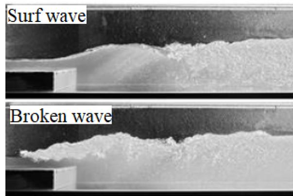
**Figure 3.** Transition from surf wave to broken wave (conventional hydraulic jump) by tailwater manipulation—photo courtesy of Wyl [33].
