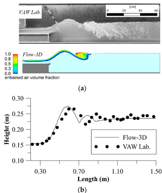
**Figure 4.** Calibration of the numerical model with laboratory data: (a) physical versus numerical simulated wave (images are at the same scale—physical model photo courtesy of Koch [24]), (b) comparison of water surface profiles.
