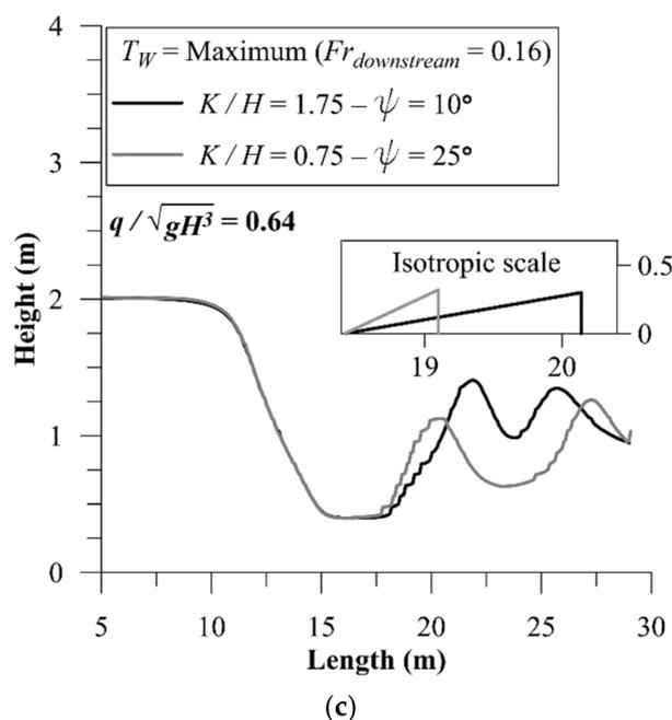
**Figure 11.** Wave adjustment by means of the kicker: (a) extremely long versus extremely steep kicker, (b) sensitivity of the extreme wave to reduction in tailwater depth, (c) extreme kickers of same height—longer versus steeper.
