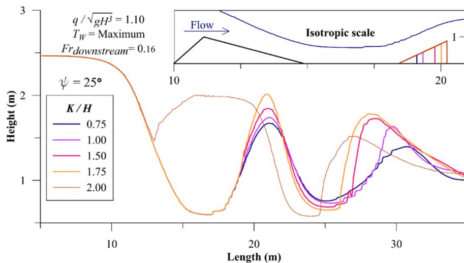
Figure 9. Effect of kicker length on wave profile.
