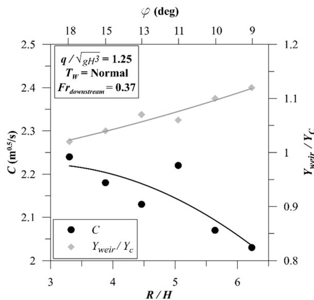
Figure 5. Weir coefficient and relative depth for ramps of different steepness.
