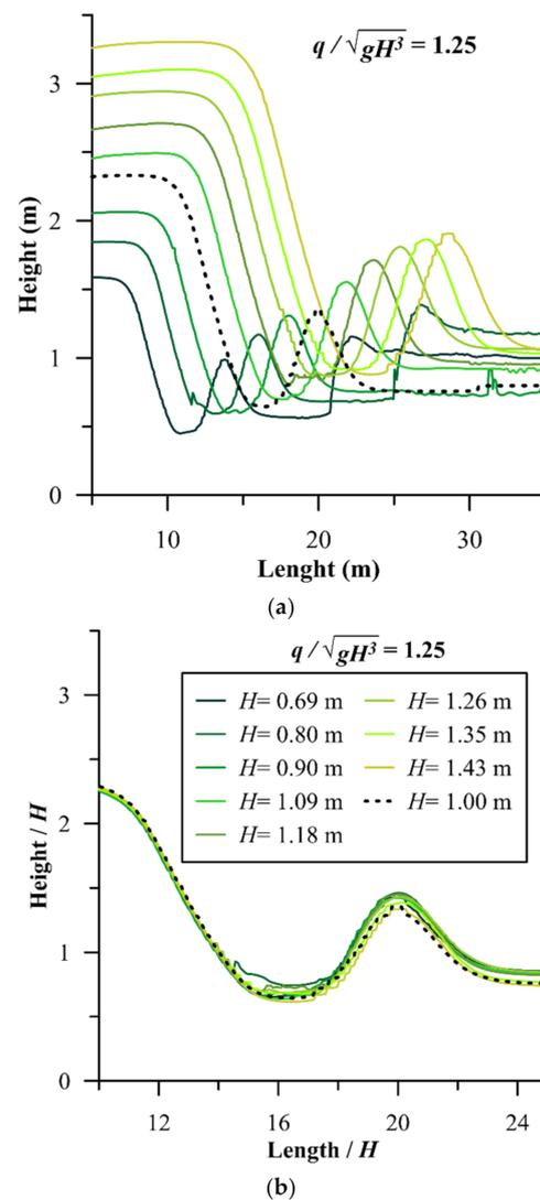
**Figure 12.** Similarity of wave profiles for ramps of different height; (a) natural dimension water surface profiles, (b) scaled (dimensionless) water surface profiles.
