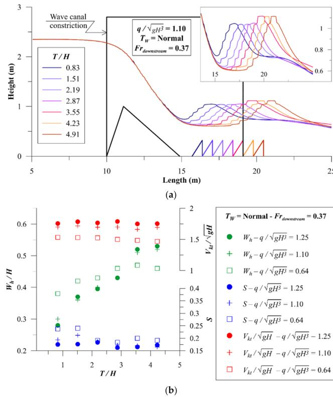
Figure 7. Effect of the transition length on the surf wave: (a) required transition for complete development of the trough, (b) sensitivity of the surf wave to transition length.
