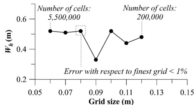
**Figure 2.** Variation of the wave height versus grid size of the computational mesh. (flow per unit width of the ramp =  $3.5 \text{ m}^2/\text{s}$ , tailwater depth =  $0.86 \text{ m}$ , ramp height =  $1.0 \text{ m}$ , Kicker length =  $0.75 \text{ m}$ , kicker angle =  $25^\circ$ ).
