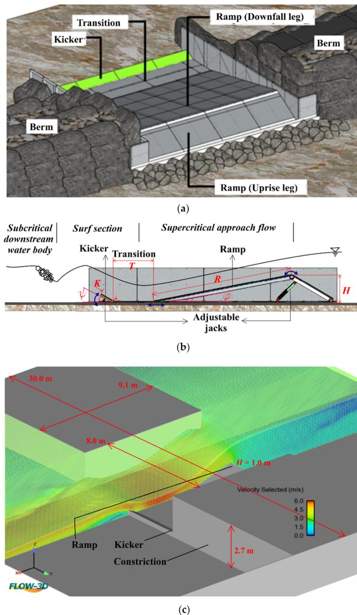
**Figure 1.** Structure under investigation: (a) perspective, (b) profile, (c) geometry of the numerical model (this does not show the full model extent to the upstream and downstream boundaries).
