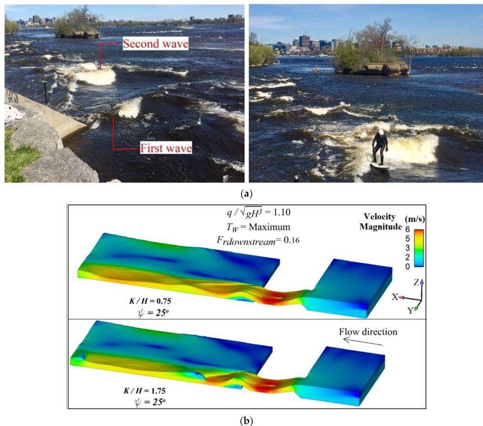
**Figure 10.** Flow field of river surf waves: (a) wave train in Ottawa river, (b) effect of kicker length on velocity field—cutaway view down the channel centerline.
