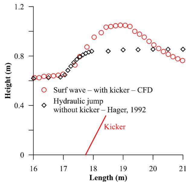
**Figure 13.** Comparing surf wave (with kicker) versus hydraulic jump (without kicker).
