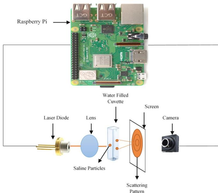
**Figure 1.** Schematic representation for determining the scattering image pattern.
