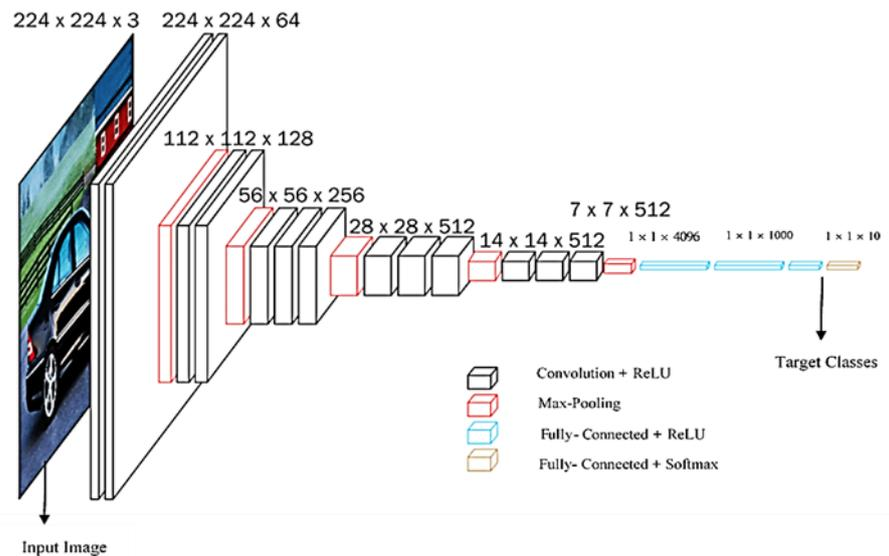
**Figure 2.** The architecture of the fine-tuned VGG-16 model.
