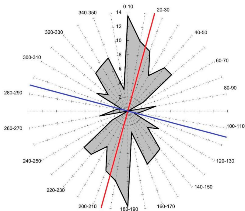
**Figure 8.** Rose diagram of the lineaments in the Ouagadougou sector. The directions shown in red (N 15) and blue (N 105) correspond to those obtained when maximising and minimising differences of the directional variograms, respectively (modified from Ouandaogo-Yaméogo (2008) [24]).
