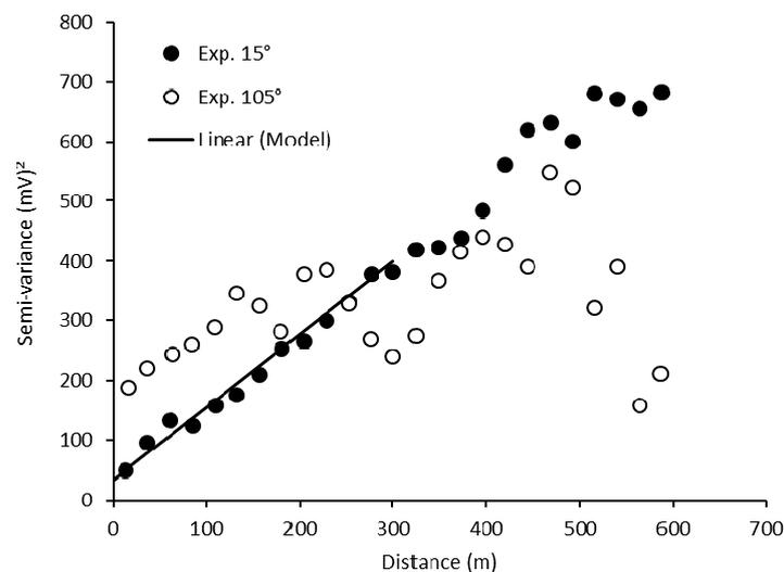
**Figure 5.** Experimental directional variogram at  $15^\circ$  and  $105^\circ$ , and fitted linear model.
