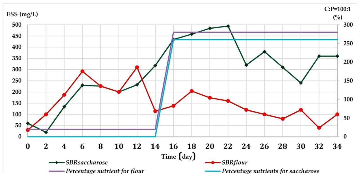
**Figure 9.** Effluent-suspended solids (ESS) with nutrient deficit (1 to 12 days) and optimal nutrient ratio (13 to 35 days) for each reactor.
