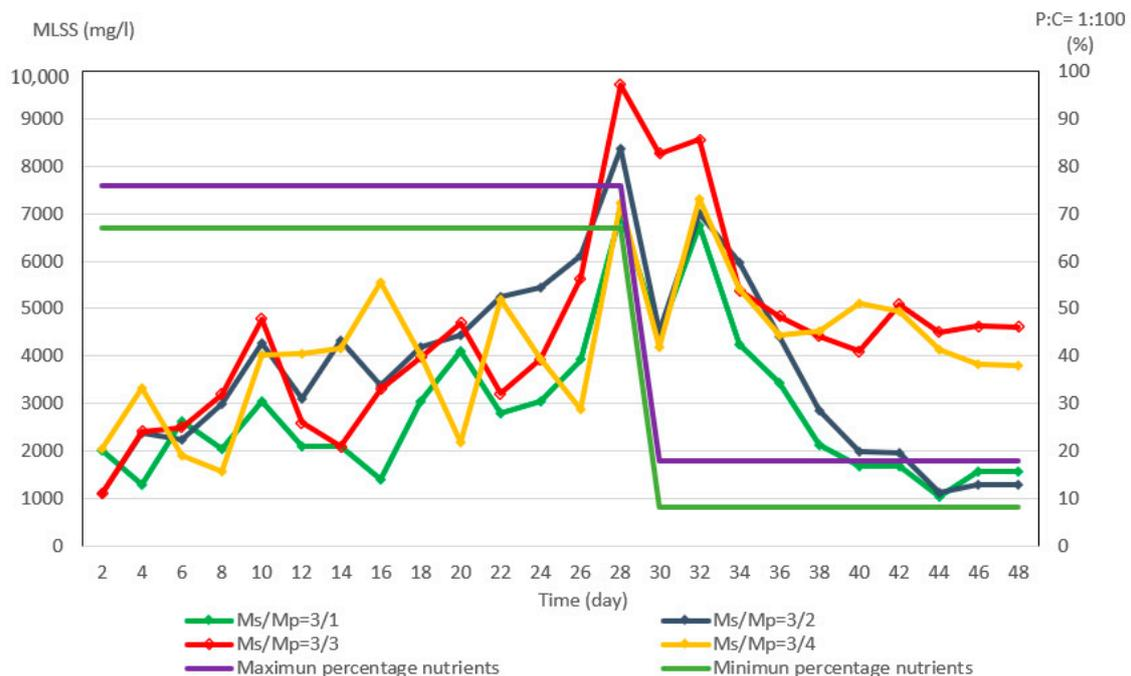
**Figure 2.** MLSS with 30% nutrient deficiency (from 1 to 30 days) and absence of nutrients (from 31 to 48 days) for each react.
