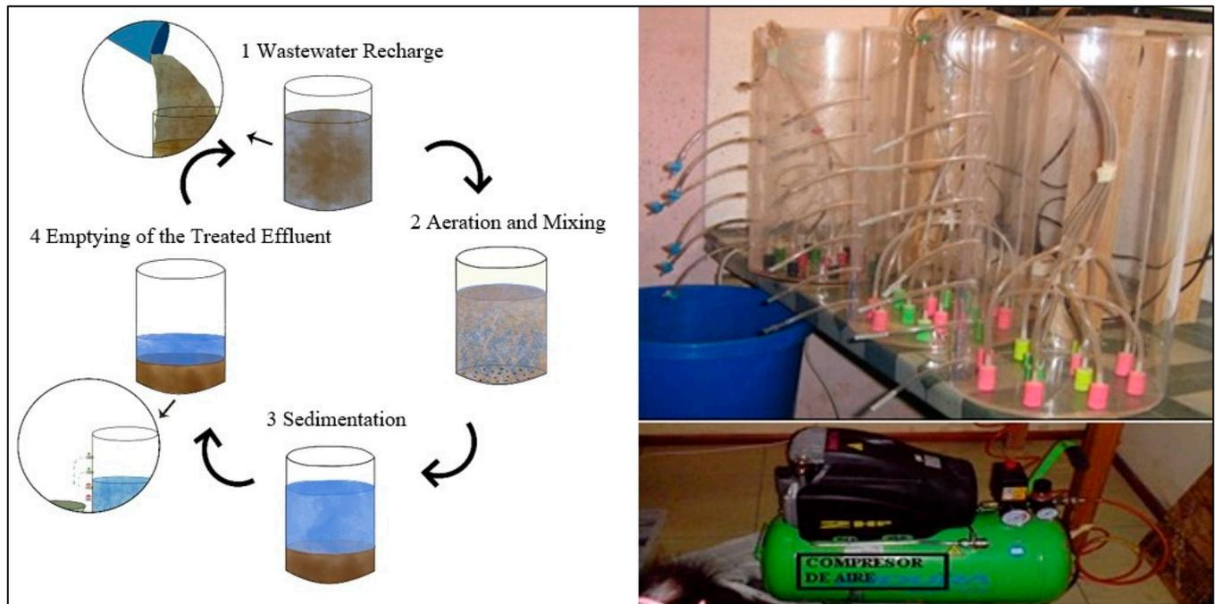
**Figure 1.** Bench Scale Activated Sludge Reactors 1. Wastewater recharge: loading raw wastewater to SBR, 3 min. 2. Aeration and mixing: compressor feeds air to SBRs, 18 h. 3. Sedimentation: separation of the aqueous and solid phases, 5 h 42 min. 4. Emptying of the treated effluent, 15 min.
