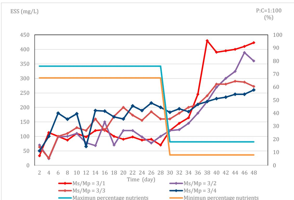
**Figure 4.** Effluent suspended solids (ESS) with 30% nutrient deficiency (from 1 to 30 days) and absence of nutrients (from 31 to 48 days) for each reactor.
