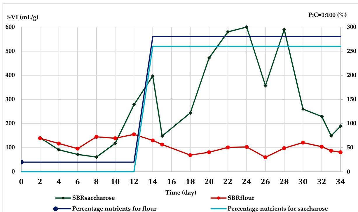
**Figure 8.** Sludge volume index (SVI) with nutrient deficit (from 1 to 12 days) and optimal ratio of nutrients (from 13 to 34 days) for each reactor.
