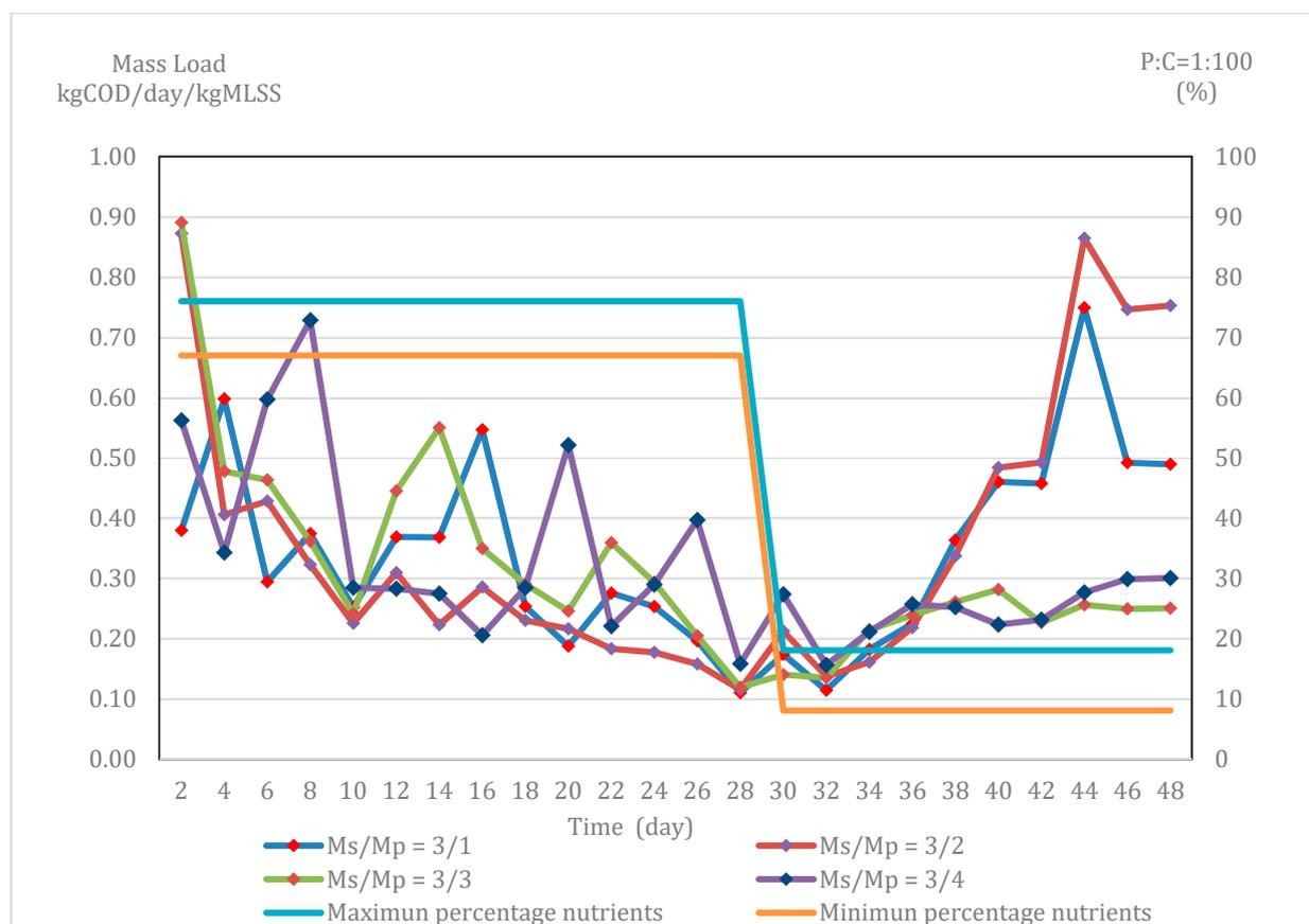
**Figure 5.** Mass Load (ML) with 30% nutrient deficiency (from 1 to 30 days) and absence of nutrients (from 31 to 48 days) for each reactor.
