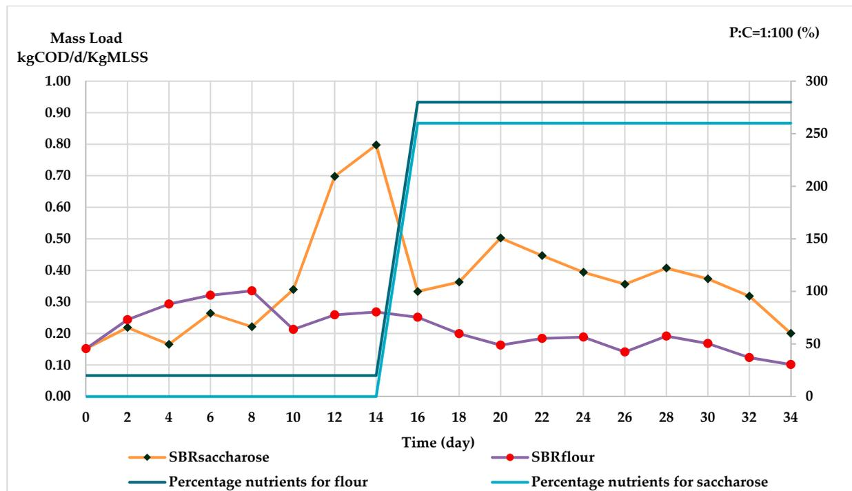
Figure 10. Mass Load (ML) with nutrient deficit (1 to 12 days) and optimal nutrient ratio (13 to 35 days) for each reactor.
