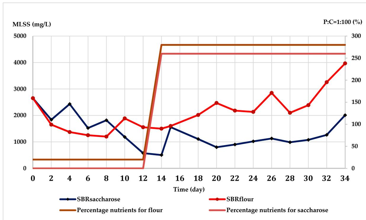
**Figure 6.** Mixing liquor-suspended solids (MLSS) with nutrient deficiency (1 to 12 days) and optimal nutrient ratio (13 to 35 days) for each reactor.
