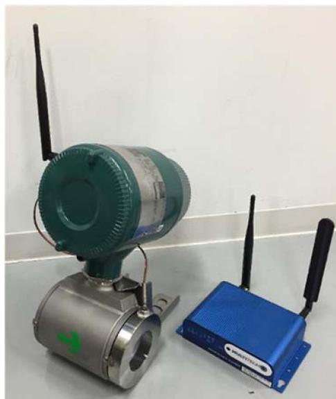
**Figure 2.** Photograph of the hot spring monitoring device.
