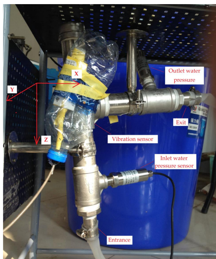
Figure 17. Schematic diagram of the subsea tree experiment assembly.
