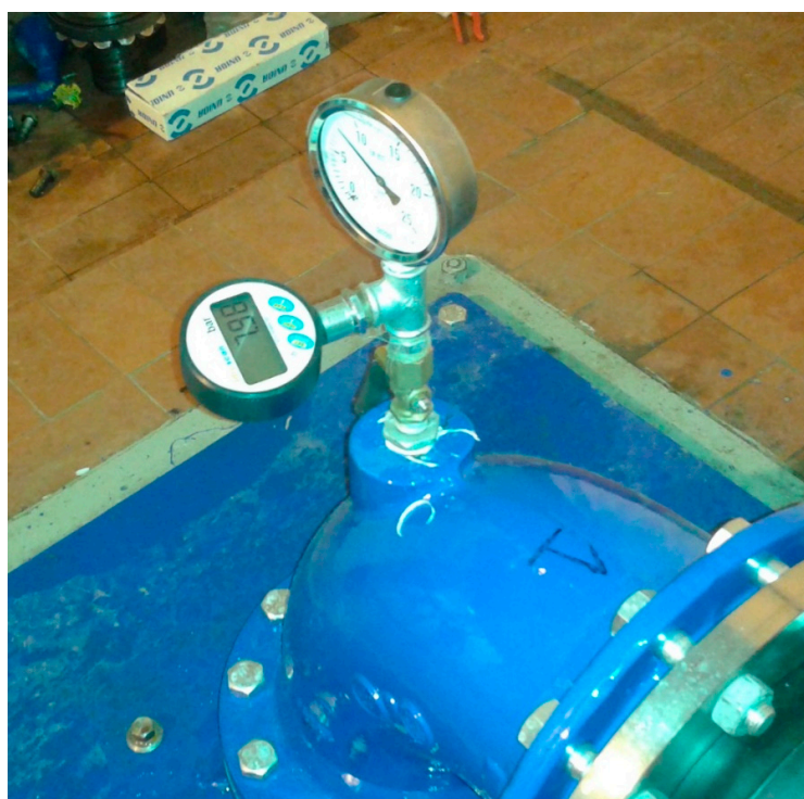
Figure 7. IDROSCAN digital manometer together with the analogue manometer.
