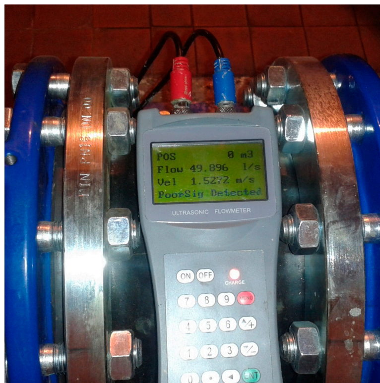
Figure 9. Portable ultrasonic flowmeter TDSH100.
