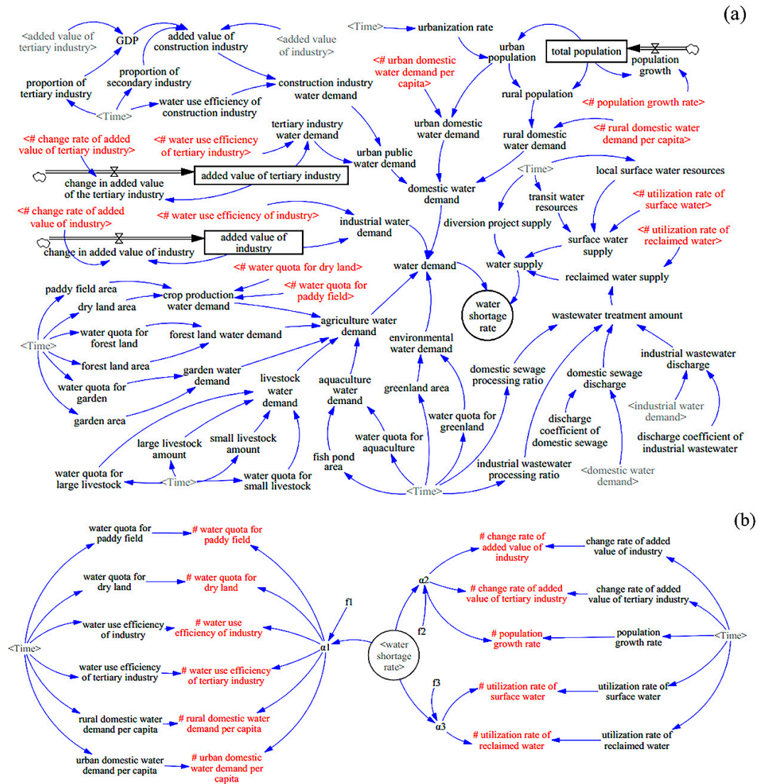
Figure 2. System flow diagrams of (a) the water supply and demand prediction module and (b) the dynamic adjustment module based on feedback. Red fonts indicate the policy adjustable variables.
