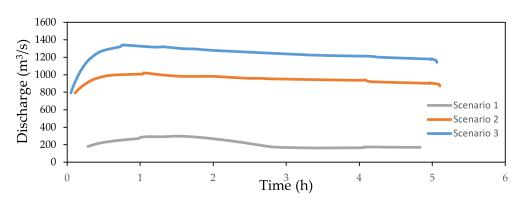
Figure 10. Dam-break flood flow curve under scenarios 1, 2, and 3.
