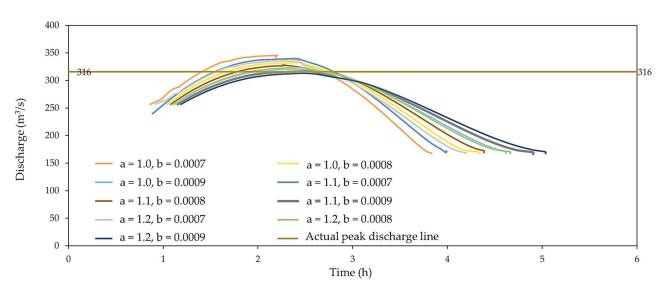
Figure 8. Simulated flow curve for the actual situation (S0) under different indices.
