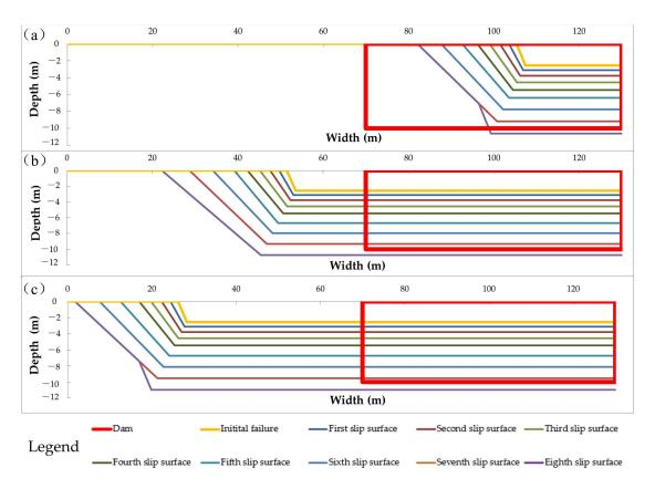
indicates that the erosion rate of the dam body gradually increased as the inflow of the barrier lake increased.
