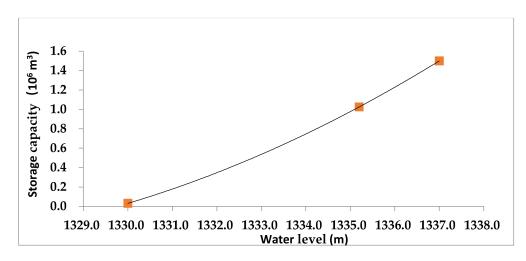
Figure 7. Barrier lake water level versus storage capacity.
