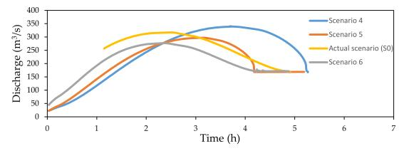
Figure 11. Flow curve of scenarios 4, 5, and 6, and the actual scenario (S0).
