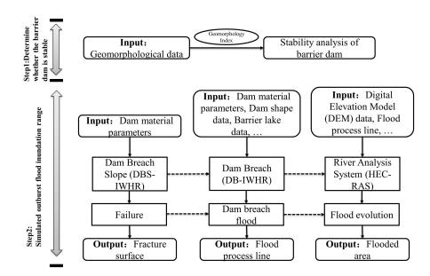
**Figure 6.** Analysis flow chart of barrier dam failure. DBS-IWHR and DB-IWHR are the abbreviations of China Institute of Water Resources and Hydropower Research's Dam Breach Slope and China Institute of Water Resources and Hydropower Research's Dam Breach, respectively. HEC-RAS represents Hydrologic Engineering Center's River Analysis System. DEM stands for Digital Elevation Model.
