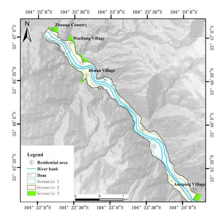
Figure 12. Flooding range map for scenarios 1, 2, and 3.
