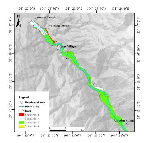
Figure 13. Inundation range of floods under different spillways.
