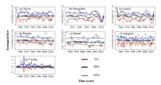
Figure 15. Centile curves of nonstationary ecological instream flow with climate factors.
