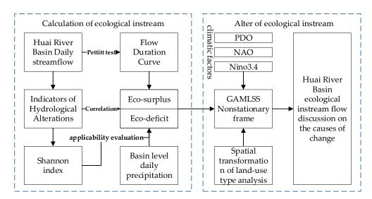
Figure 2. Working procedure for the calculation and change of ecological instream flow.
