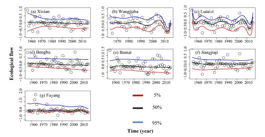
Figure 14. Centile curves of stationary ecological instream flow.
