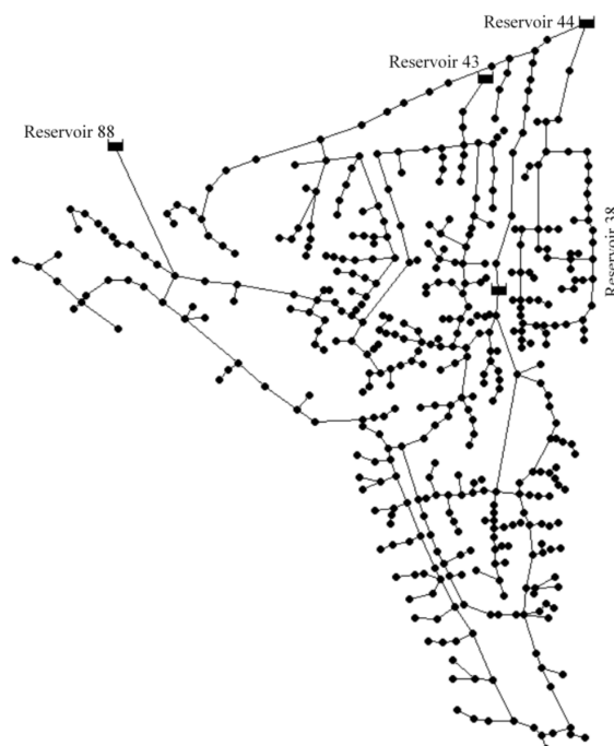
Figure 2. Schematic of the Balerma Network (Test Problem 1).
