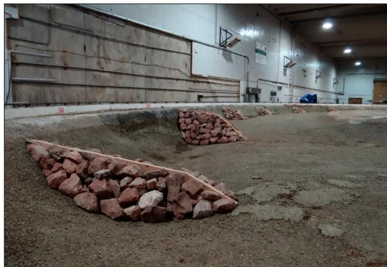
Figure 7. Constructed installation of rock vanes (looking downstream) [21]. Plywood in the center of each structure is used for impermeability.
