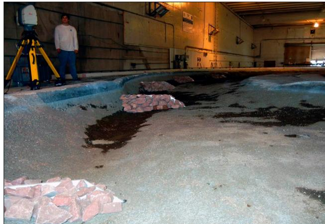
**Figure 8.** Bendway weir configuration looking downstream [23]. Plywood in the center of each structure is used for impermeability.
