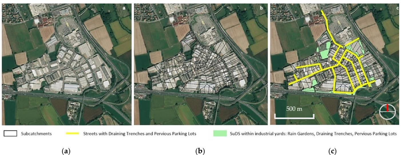
**Figure 4.** Catchment C (a), subdivision into subcatchments (b), and SuDS distribution within the subcatchments (c).
