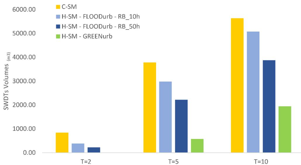
**Figure 8.** Stormwater detention tanks total volumes: a comparison between the investigated C-SM and H-SM scenarios.
