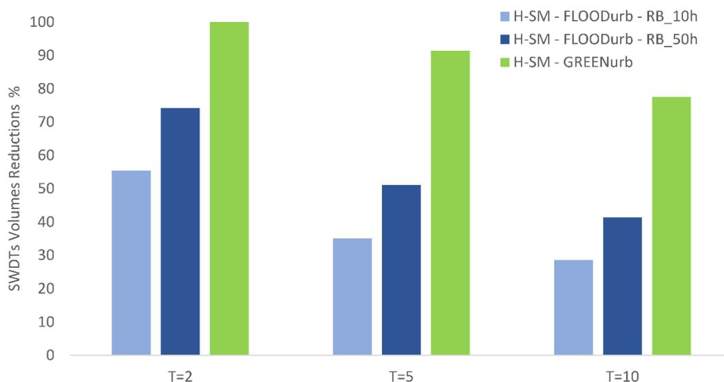
**Figure 9.** Mean reductions of stormwater volumes to be discharged into SWDTs (D).
