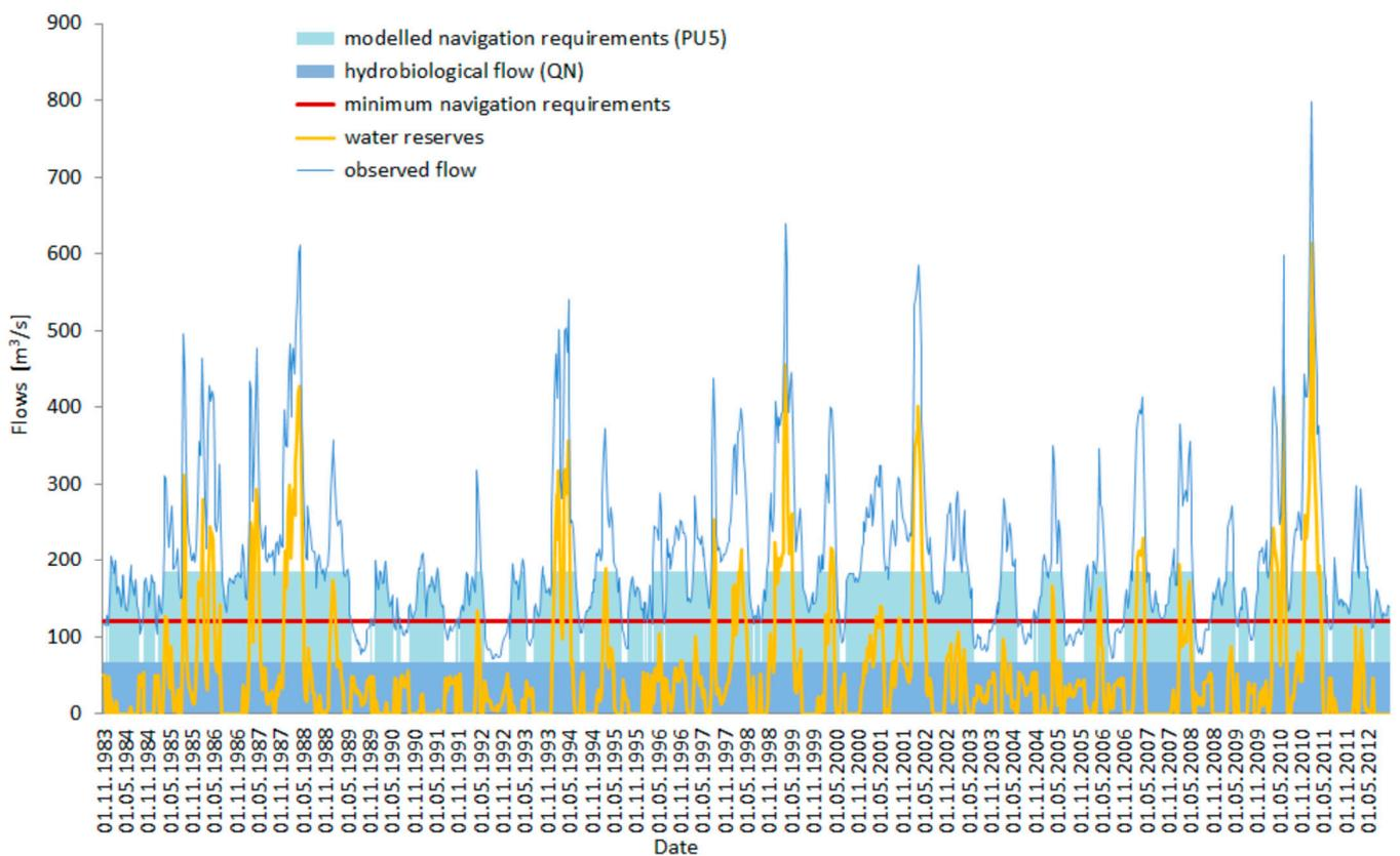
**Figure 2.** Balance flows of the Warta River at the cross-section PB5 with appraisal of the navigation conditions and water reserves.
