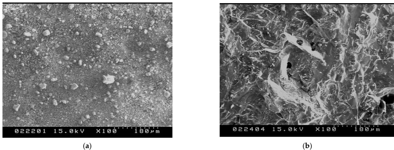
**Figure 2.** Results of SEM analysis of the dust before (a) and after (b) ISV treatment.
