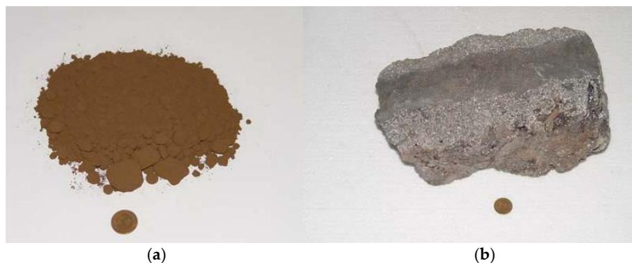
**Figure 1.** Exterior of the dust before (a) and after (b) ISV treatment.
