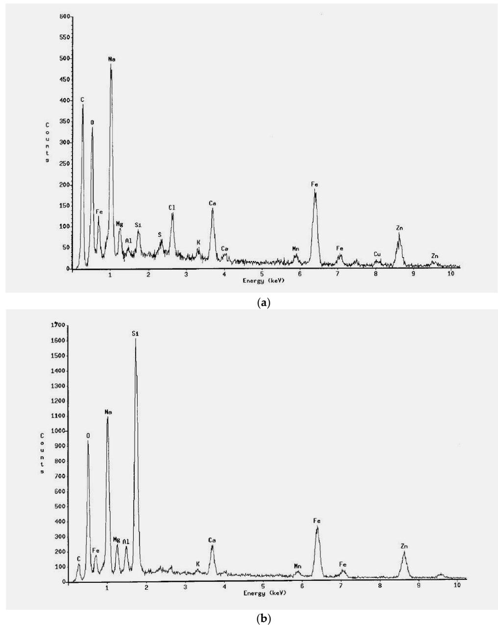
**Figure 3.** Results of EDS analysis of the dust before (a) and after (b) ISV treatment.
