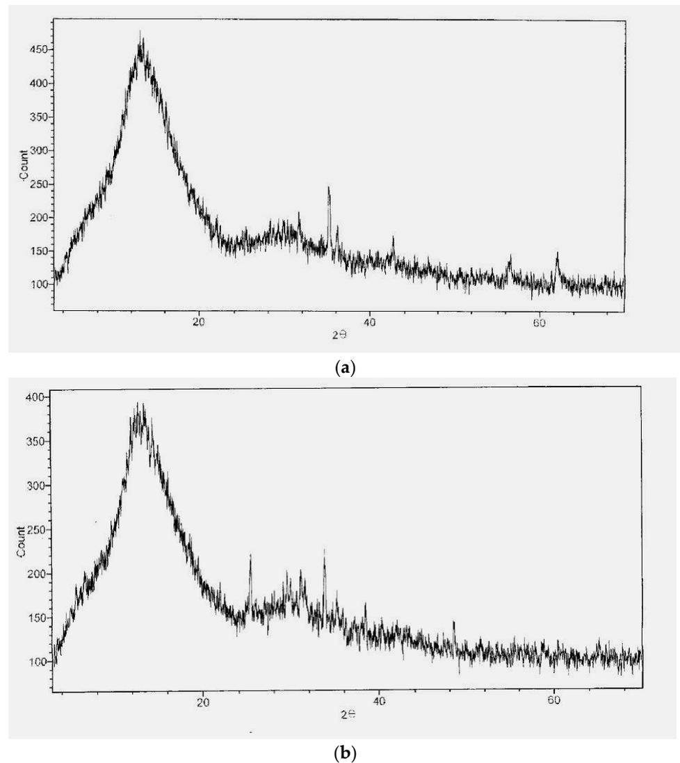
**Figure 4.** Results of XRD analysis of the dust before (a) and after (b) ISV treatment.
