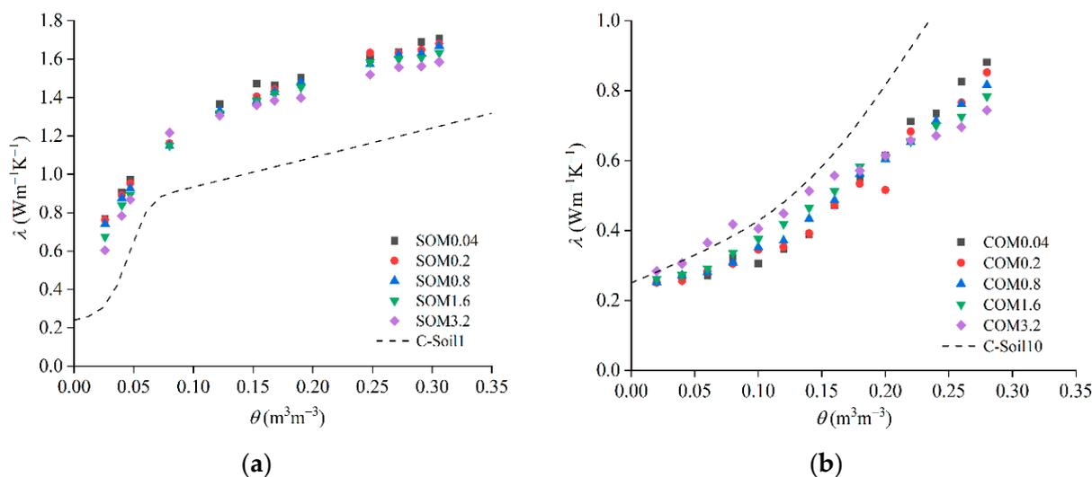
**Figure 3.** The relationship of  $\lambda \sim \theta$  and the curve estimated by the Campbell model for soil with different organic matter contents. Figure (a) shows the results of Soil 1, representing sandy soil. Figure (b) shows the results of Soil 10, representing clay soil.
