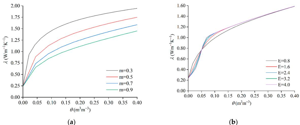
**Figure 4.** The influence of m and E values on the shape of the  $\lambda$ - $\theta$  curve, respectively. Figure (a) shows the influence of different values of m on the curve when  $E = 0.8$  and Figure (b) shows the influence of different values of E on the curve when  $m = 0.7$ .
