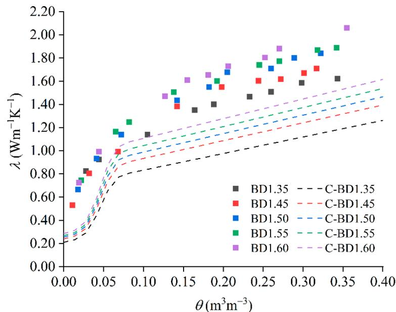
**Figure 2.** The measured relationship of  $\lambda$ – $\theta$  and the curves estimated by the Campbell model for soil with different bulk densities. The colored dots represent the measured values and the dotted lines represent the Campbell model curves.
