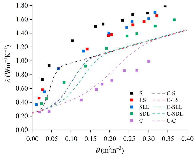
**Figure 1.** The measured relationship of  $\lambda \sim \theta$  and the curves estimated by the Campbell model for soil with different textures. The colored dots represent the measured values and the dotted lines represent the Campbell model curves.
