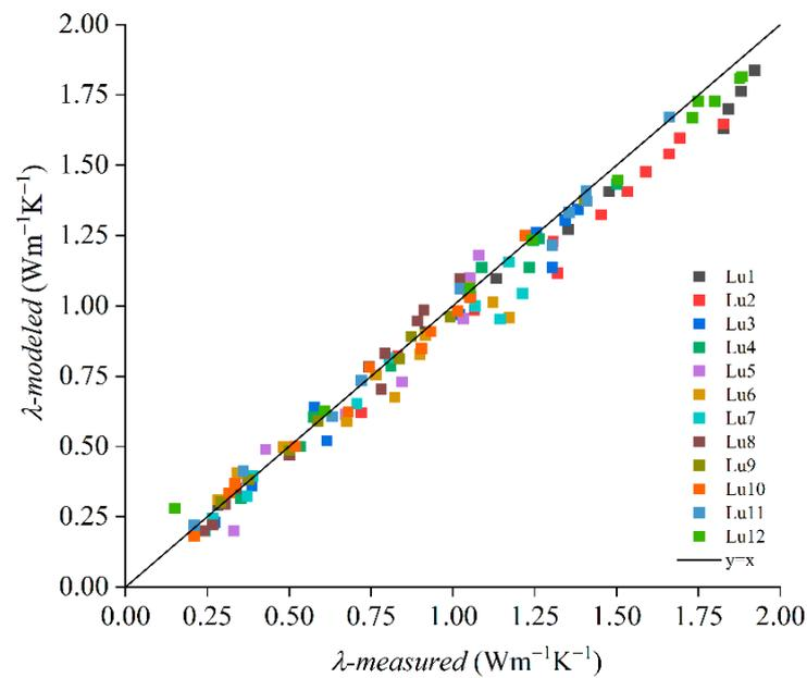
Figure 6. Comparison of soil thermal conductivity predicted from the revised model vs. measured values.
