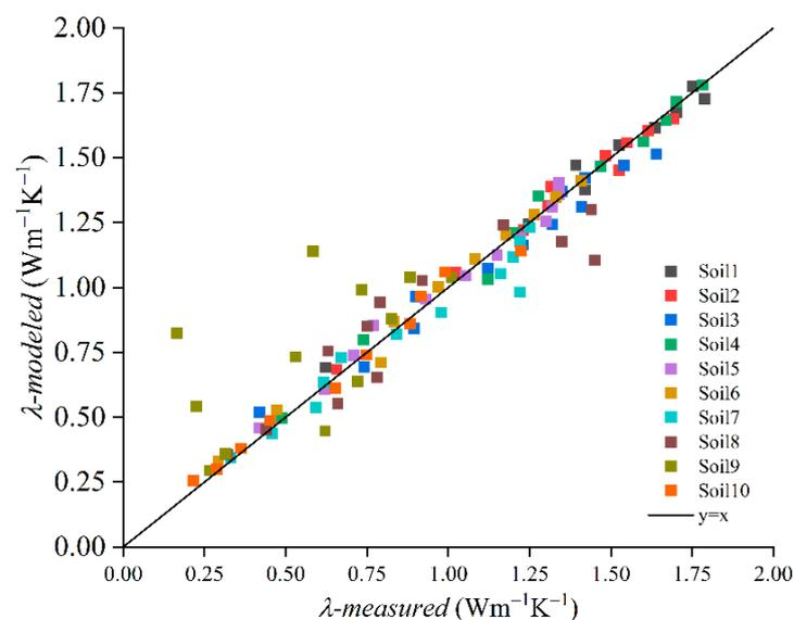
**Figure 5.** Comparison of predicted soil thermal conductivity ( $\lambda$ ) values from the new model vs. measured data under the same water content of soils in Table 1.
