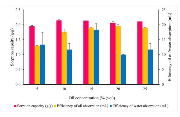
**Figure 9.** The influence of oil concentration on the sorption capacity and the efficiency of oil/water absorption by RS heat treated at 120  $^{\circ}$ C for 20 min and at the selected packing density. Error bars represent the mean  $\pm$  SEM of three replicates.
