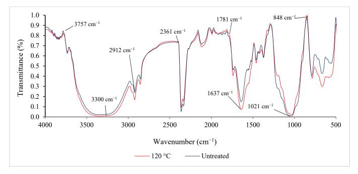
Figure 4. ATR-IR spectra of untreated and pre-treated (120 °C) RS after wetting with oil-seawater mixture.
