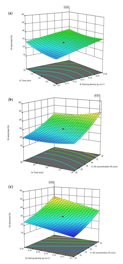
**Figure 10.** Three-dimensional contour plots generated by Design-Expert (Stat Ease, Inc) of the model terms (**a**) A: time of heating and B: packing density, (**b**) B: time of heating and C: oil concentration and (**c**) B: packing density and D: oil concentration.
