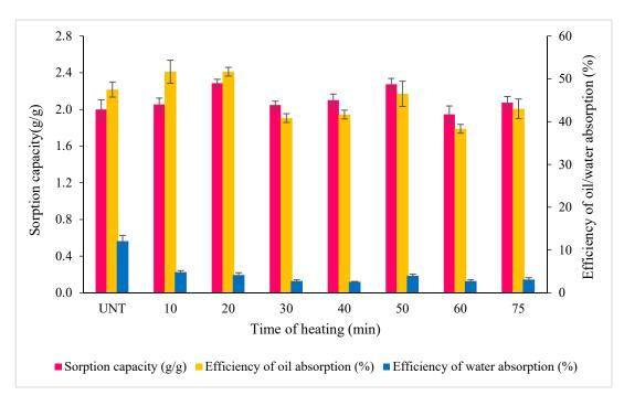
**Figure 7.** The effect of time of heating on the sorption capacity and the efficiency of oil/water absorption by RS pre-treated at 120 °C. Error bars represent the mean  $\pm$  SEM of three replicates.
