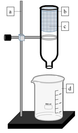
**Figure 1.** Experimental setup for the filter system: (**a**) retort stand; (**b**) plastic bottle; (**c**) cylinder holder; (**d**) beaker.
