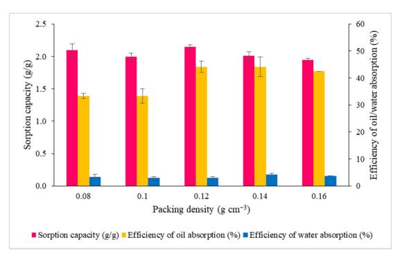
**Figure 8.** The effect of packing density on the sorption capacity and efficiency of oil/water absorption of RS pre-treated at 120 °C for 20 min. Error bars represent the mean  $\pm$  SEM of three replicates.
