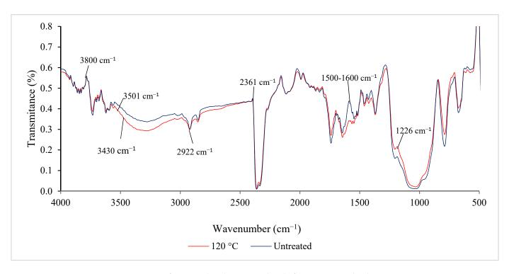
Figure 3. ATR-IR spectra of untreated and pre-treated RS before wetting with oil-seawater mixture.
