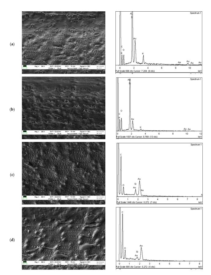
**Figure 5.** Images from scanning electron microscopy (SEM, left) and outputs of EDX (right): (**a**) untreated rice straw before wetting with oil–seawater mixture; (**b**) untreated rice straw after wetting with oil–seawater mixture; (**c**) pre-treated rice straw after wetting with oil–seawater mixture.
