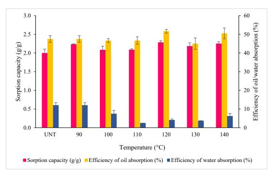
**Figure 6.** The effect of temperature pre-treatment of RS on the sorption capacity and the efficiency of oil/water absorption. Error bars represent the mean  $\pm$  SEM of three replicates.
