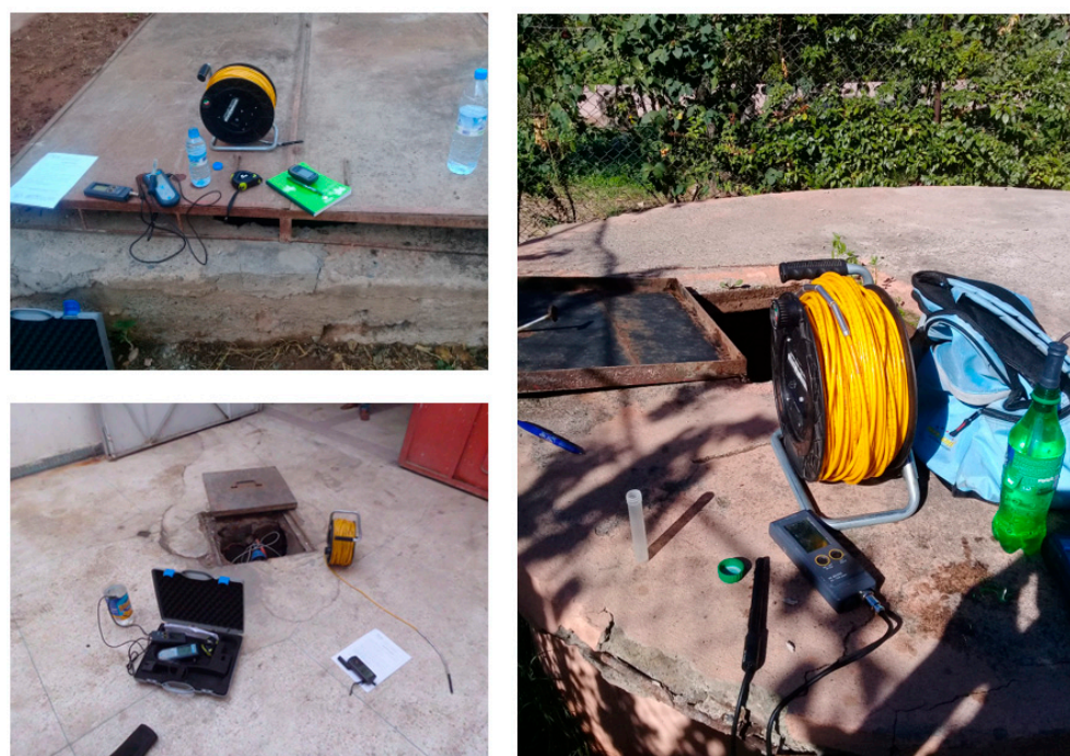
Figure 6. Example of wells prospected and equipment used for groundwater level survey.
