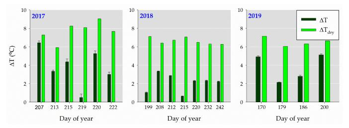
**Figure 8.** Mean  $\Delta$ T values observed during the water stress period in the deficit irrigation treatments (WS). In 2019, the first two dates correspond to the flowering stress treatment (WS1) and the last two dates to the grain-filling stress treatment (WS2). For each measurement date, the  $\Delta$ T<sub>*dry*</sub> values calculated with Equation (3) are also plotted. Each bar indicates the mean  $\pm$  s.e. of 18 (2017, 2018) and 12 (2019) maize breeding plots.
