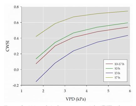
**Figure 5.** Sensitivity analysis of crop water stress index (CWSI) to four pairs of  $a_{pot}/b_{pot}$  values: (1) values derived for the period 10–17 h UTC, (2) values derived for the 10 h UTC time period, (3) values derived for the 13 h UTC time period, (4) values derived for the 17 h UTC time period. Equations (1)–(3) have been used to compute CWSI. A fixed  $\Delta$ T value of 2 °C was used in all cases.
