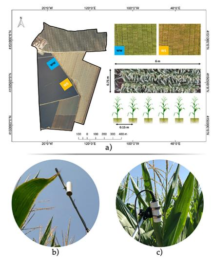
**Figure 1.** (a) Illustration of the experimental maize breeding field; (b) detail of the infrared thermometer (model IR120, Campbell Scientific Ltd., Shepshed, UK) installed on a well-watered maize plot; (c) detail of the infrared thermometer (model MI-230, Apogee Instruments Ltd., Logan, UT, USA) used for manual  $T_c$  measurements.
