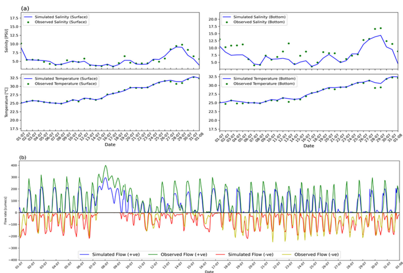
Figure 12. Comparison between simulation and observation for case 4: (a) Time series comparison of simulated salinity and water temperature upstream of Ohashi River for July 2012; (b) time series comparison of the flowrate of Ohashi River.
