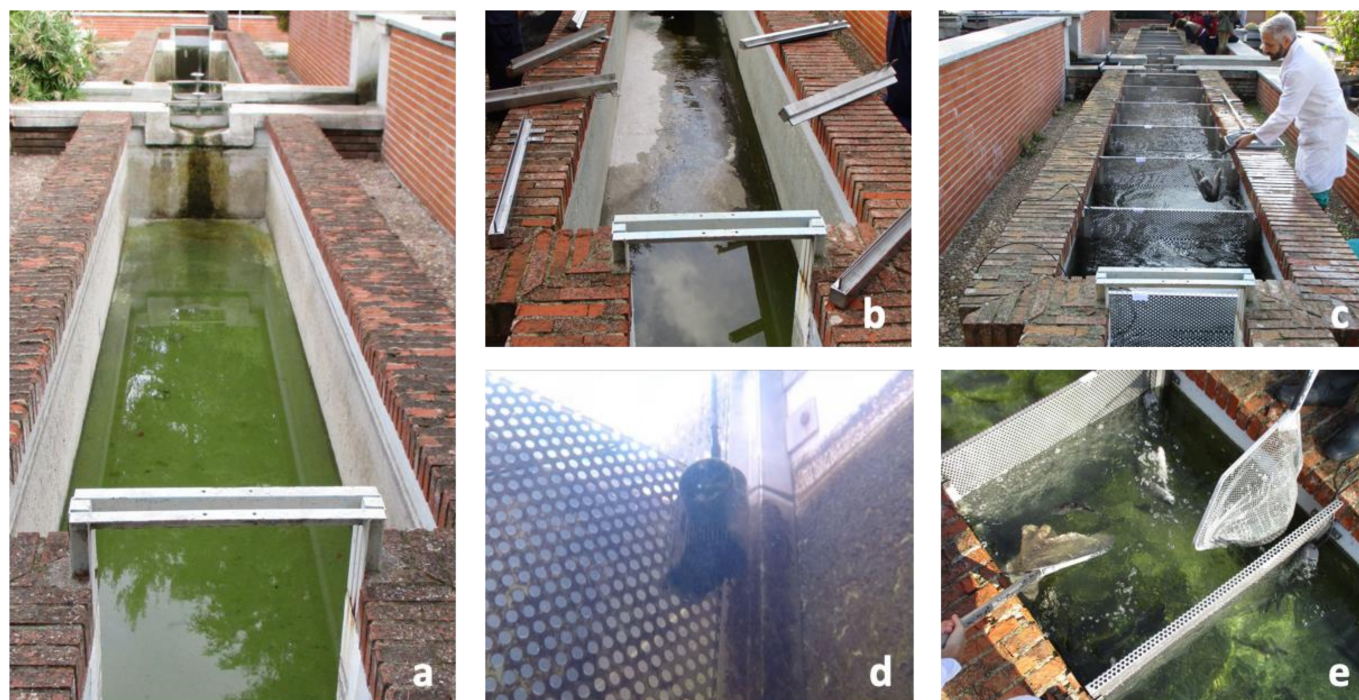
Figure 1. Different aspects of the adaptation and operation of the tanks for the study: (a) overview of the complete raceway before the study; (b) adaptation of the tank sections; (c) image of the raceway with separations with tanks; (d) underwater image of one of the water pumps used for generating under water currents; and (e) image of one tank.
