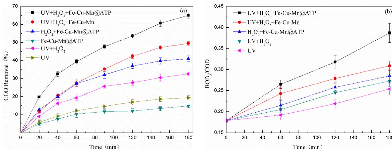
**Figure 3.** (a) COD removal and (b) BOD<sub>5</sub>/COD change of the chemical pharmaceutical wastewater by different treatment systems.
