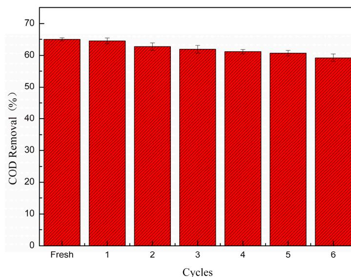
**Figure 11.** Effect of recycling the catalyst on COD removal (initial pH of 2.0; Catalyst dosage of 10.0 g/L; The concentration of  $H_2O_2$  is 0.5 mol/L; The illumination distance is 20 cm).
