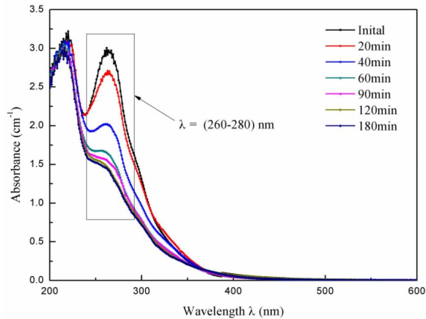
**Figure 9.** Evolution of UV-vis spectrum in catalytic oxidation of chemical pharmaceutical wastewater.
