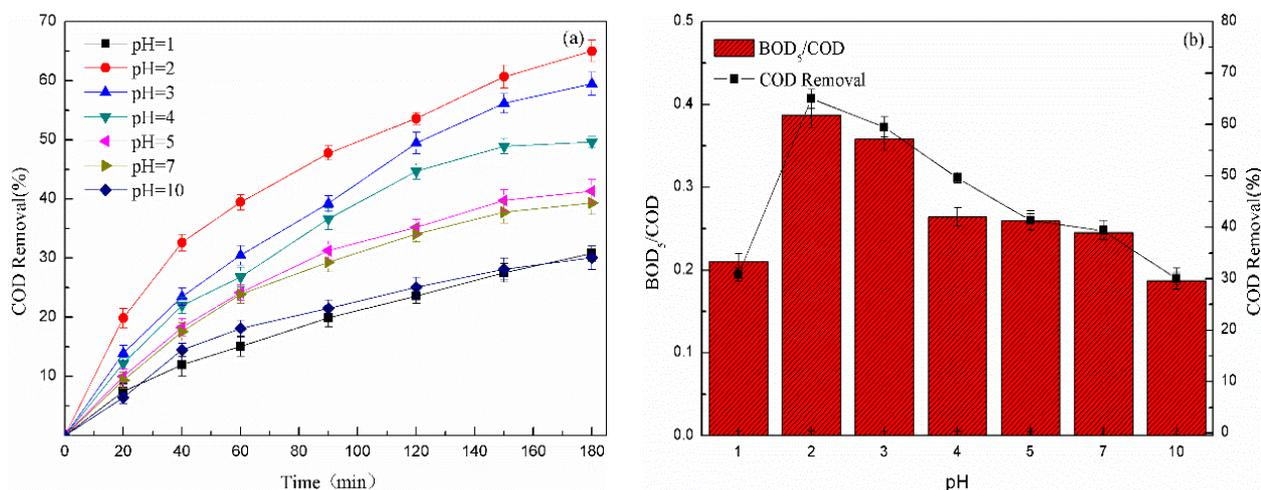
**Figure 4.** Effect of initial pH on (a) COD removal and (b)  $BOD_5/COD$  of chemical pharmaceutical wastewater (Fe-Mn-Cu@ATP dose = 10.0 g/L, hydrogen peroxide concentration = 0.5 mol/L, light distance = 20 cm).
