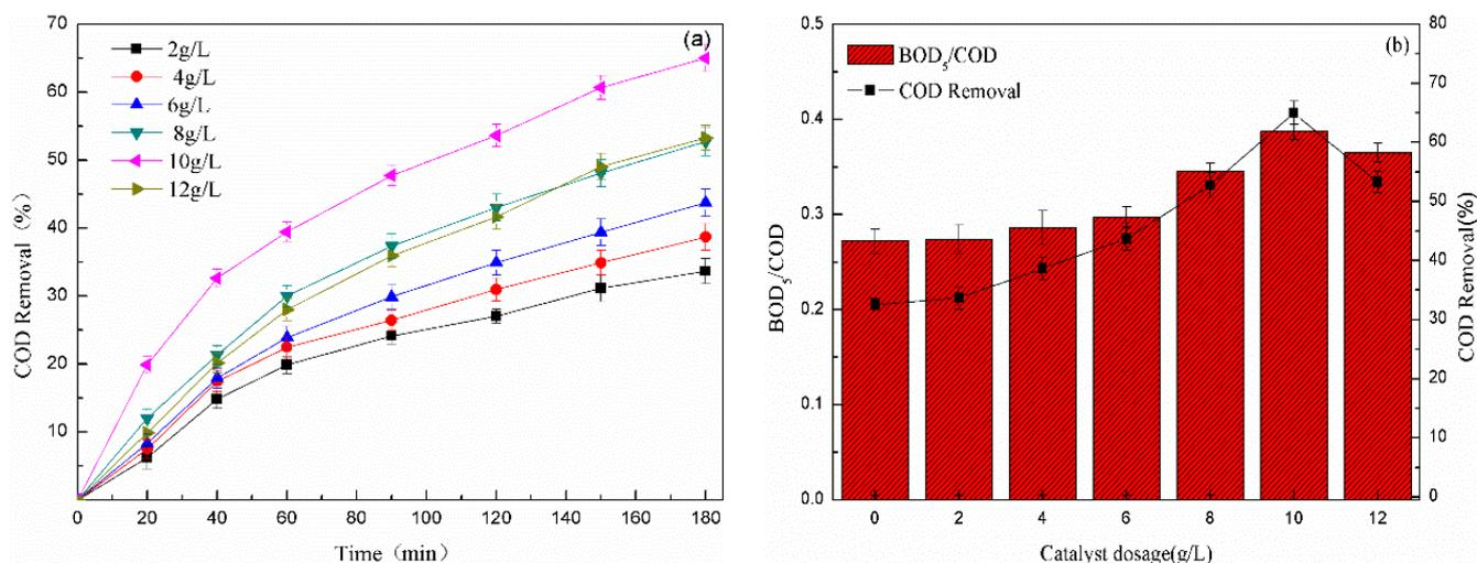
**Figure 5.** Effect of catalyst dosage on (a) COD removal and (b) BOD<sub>5</sub>/COD of pharmaceutical wastewater (initial pH = 2.0, hydrogen peroxide concentration = 0.5 mol/L, light distance = 20 cm).
