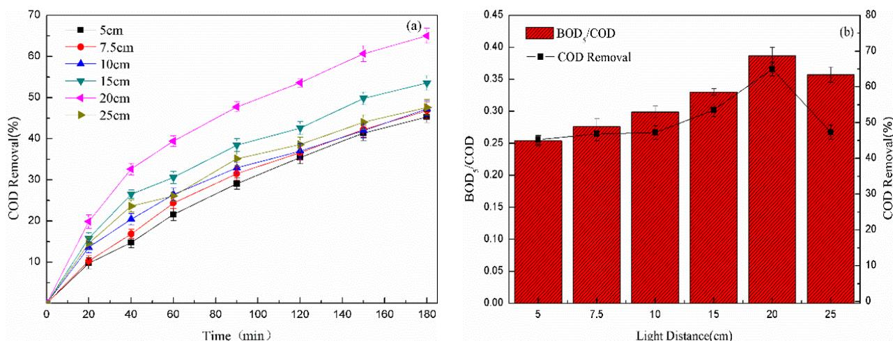
**Figure 7.** Effect of light distance on (a) COD removal and (b) BOD<sub>5</sub>/COD of pharmaceutical wastewater (initial pH = 2.0, hydrogen peroxide dosage = 0.5 mol/L, light distance = 20 cm).
