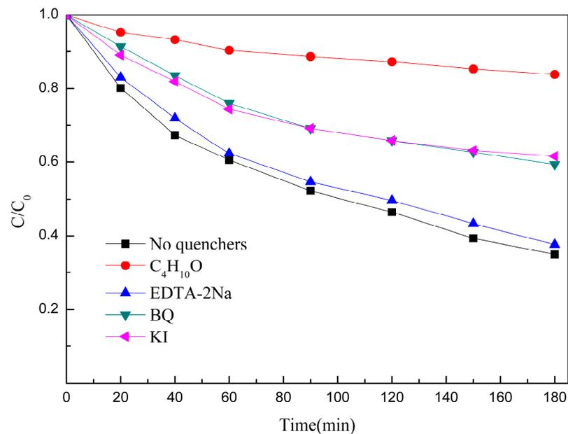
**Figure 10.** Effects of different group capture factors on COD removal of pharmaceutical wastewater.
