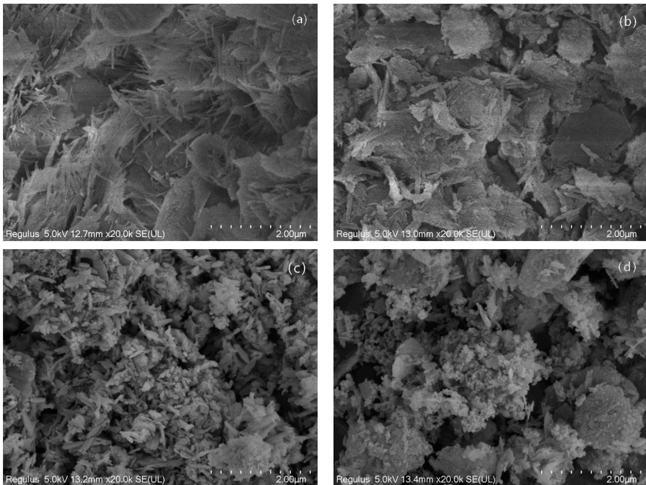
**Figure 2.** SEM photographs of (a) acid modified attapulgite (ATP), (b) Acid modified ATP, (c) Fe-Mn-Cu and (d) Fe-Mn-Cu@ATP.
