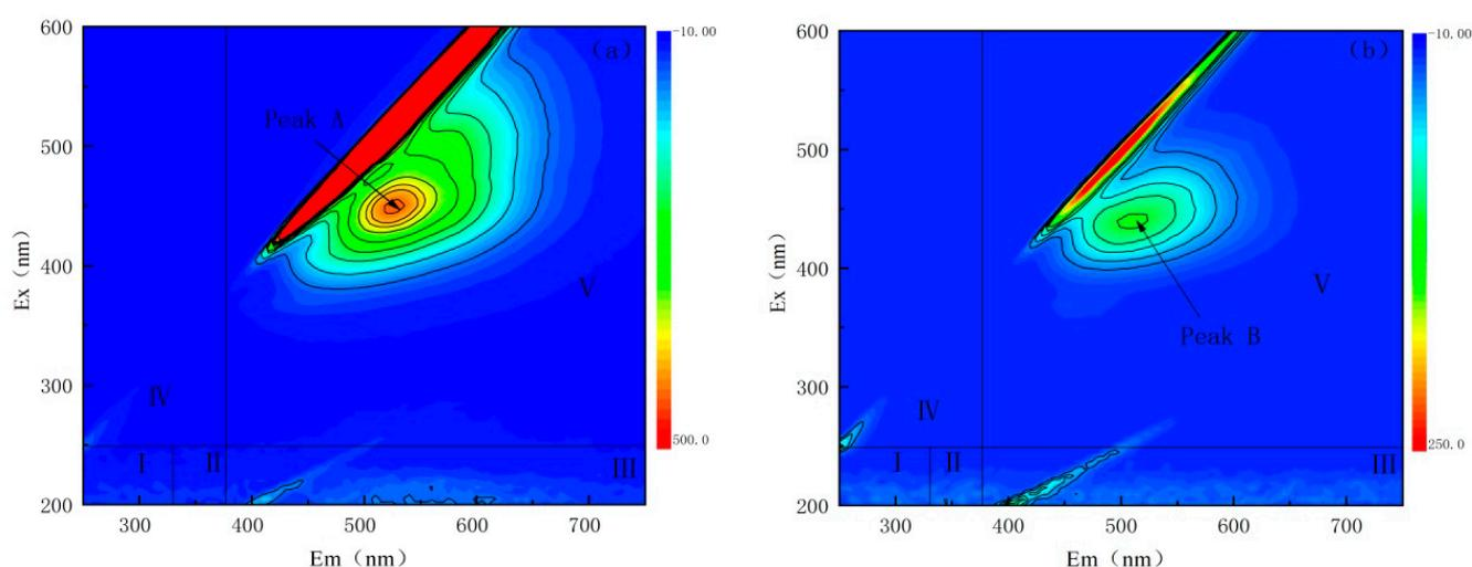
**Figure 8.** 3D-excitation emission matrix fluorescence spectroscopy of (a) input pharmaceutical wastewater and (b) treated pharmaceutical wastewater.
