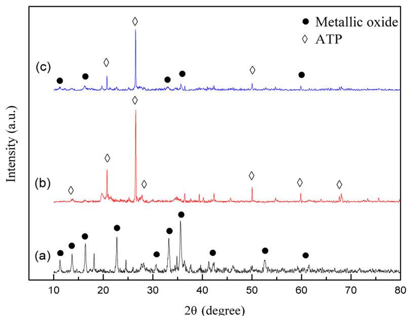
**Figure 1.** X-ray diffraction (XRD) patterns of (a) Fe-Mn-Cu, (b) ATP and (c) Fe-Mn-Cu@ATP.
