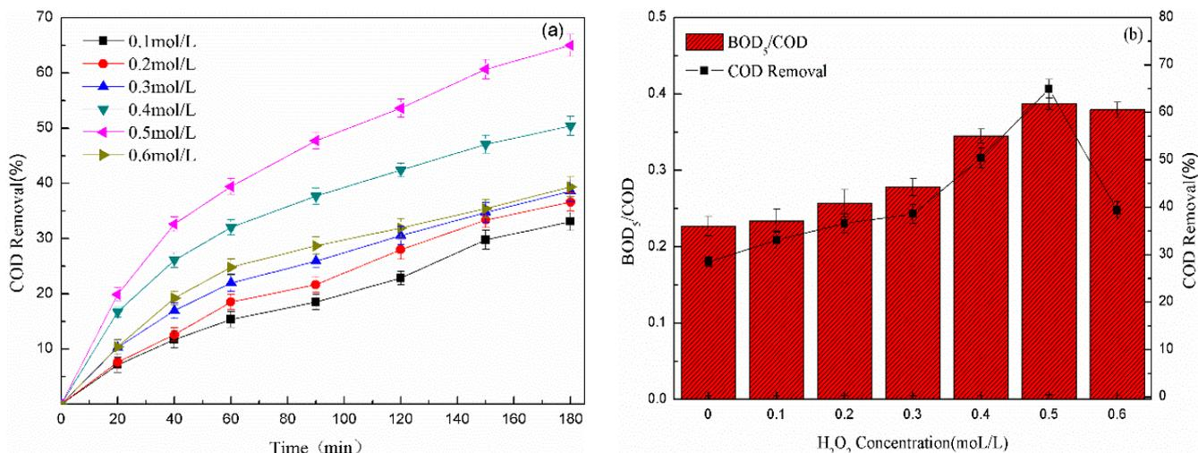
**Figure 6.** Effect of H<sub>2</sub>O<sub>2</sub> concentration on (a) COD removal and (b) BOD<sub>5</sub>/COD of pharmaceutical wastewater (initial pH = 2.0, catalyst dosage = 10.0 mol/L, light distance = 20 cm).
