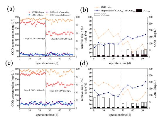
**Figure 1.** Organic matter removal and the  $COD_{intra}$ ,  $COD_{dn}$  and  $SND_{ratio}$  in SNDPR system with different COD concentrations in influent. ((a,b): 100 kPa; (c,d,b): 72 kPa).
