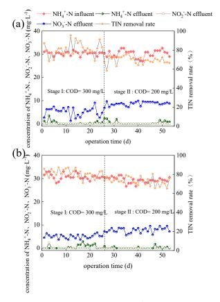
**Figure 2.** Variations of influent  $NH_4^+$ -N, effluent  $NH_4^+$ -N,  $NO_2^-$ -N and  $NO_3^-$ -N and TIN removal efficiency under different COD in influent ((a): 100kPa, (b): 72 kPa).
