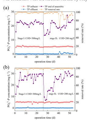
**Figure 3.** Removal of  $PO_4^{3+}$ -P in a SNDPR system under different COD concentrations in influent ((a): 100 kPa, (b): 72 kPa).
