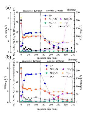
**Figure 4.** Variations of N, P and organic carbon in cyclic study in stage II (COD = 200 mg/L) ((a): 100 kPa, (b): 72 kPa).
