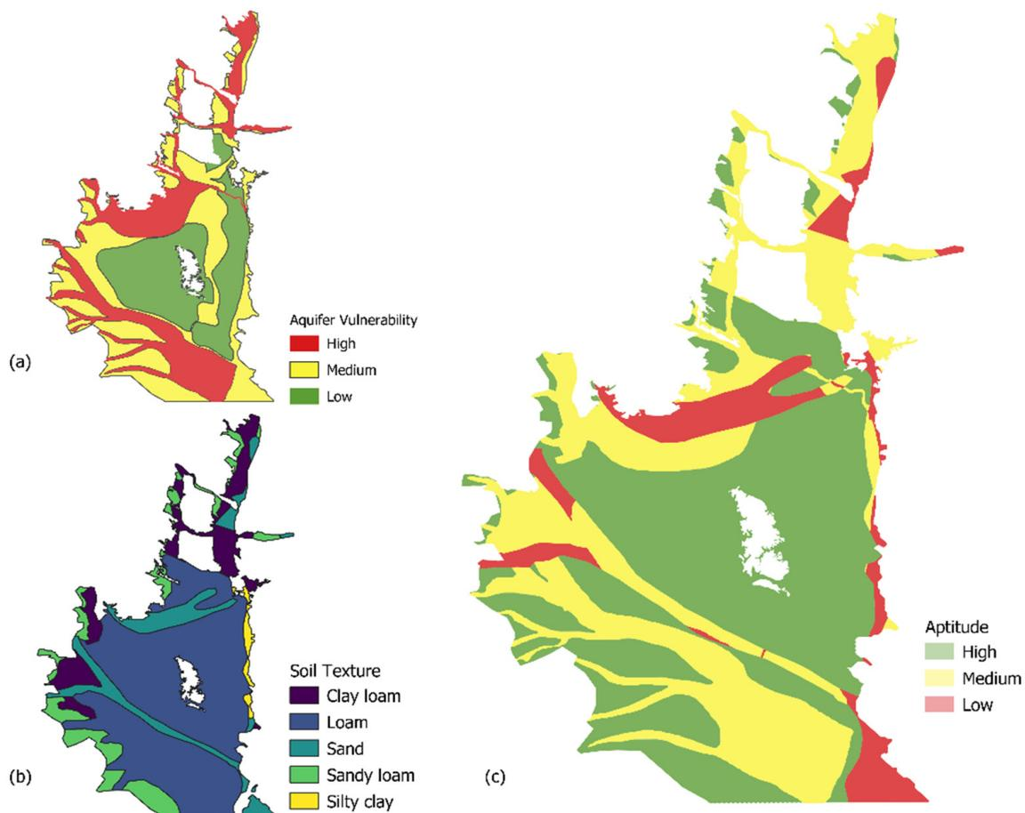
**Figure 4.** Aptitude map for ODWTS combining Environmental factors. (a) Aquifer vulnerability; (b) Soil texture; (c) Aptitude map for ODWTS installation.
