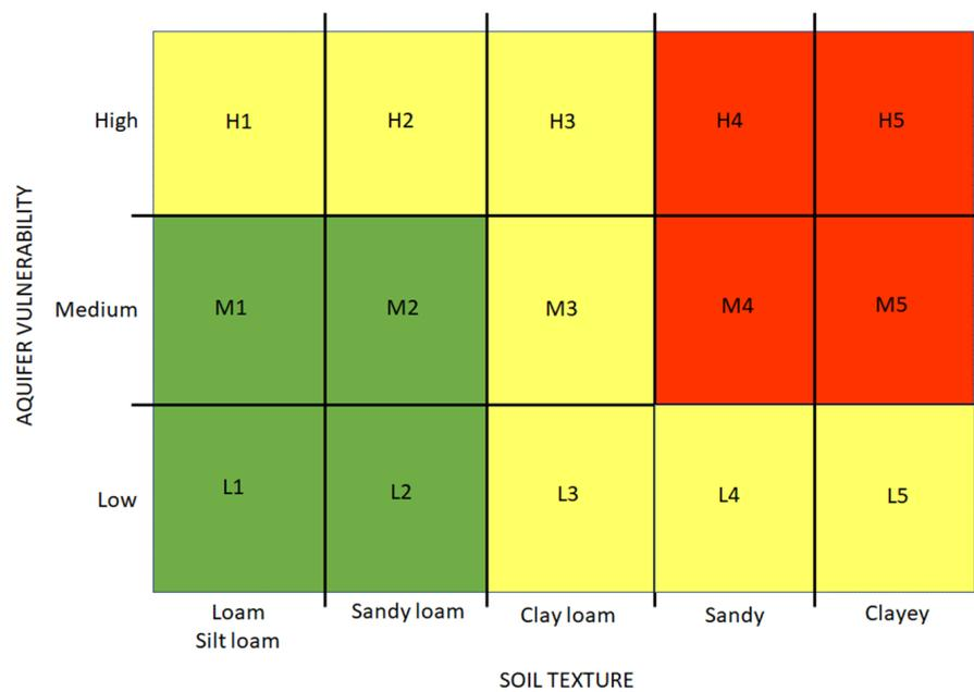
**Figure 3.** Possible combinations between soil texture and aquifer vulnerability categories. Green: acceptable aptitude for ODWST, Yellow: further examination is needed, Red: no suitable for ODWTS. The codification of Aptitude factors is described in detail in Table 1.
