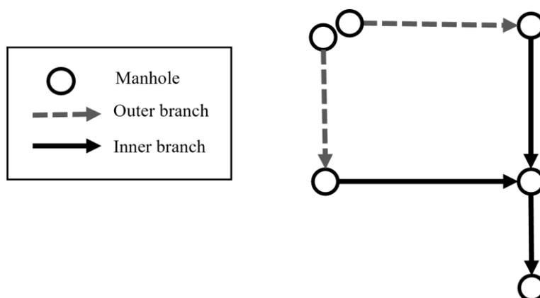
Figure 1. Types of pipes in the sewer network.
