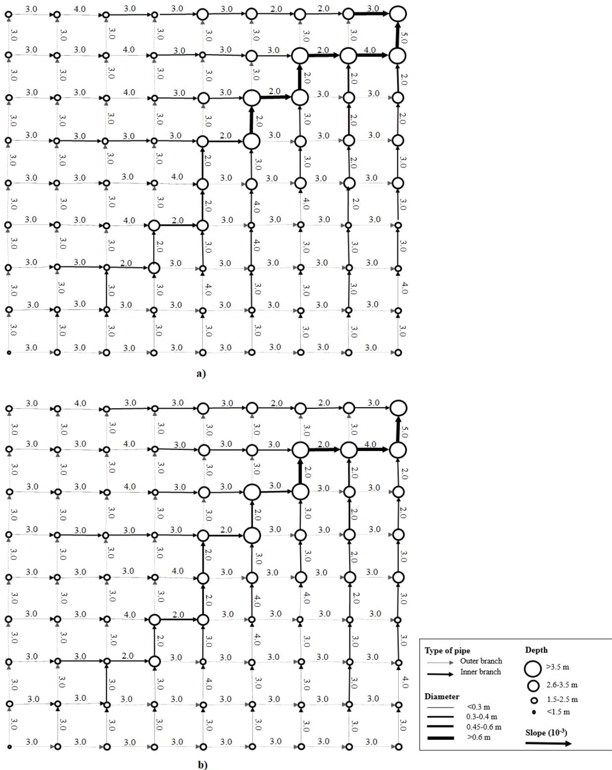
**Figure 7.** Scheme (not to scale) of the best design of the benchmark network proposed by Moeini and Afshar [46] with (a) the cost function of Li and Matthew [34] and (b) the cost function of Maurer et al. [47].
