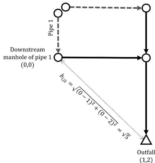
Figure 4. Example of the calculation of  $b_{ijt}$  with Criterion 3.
