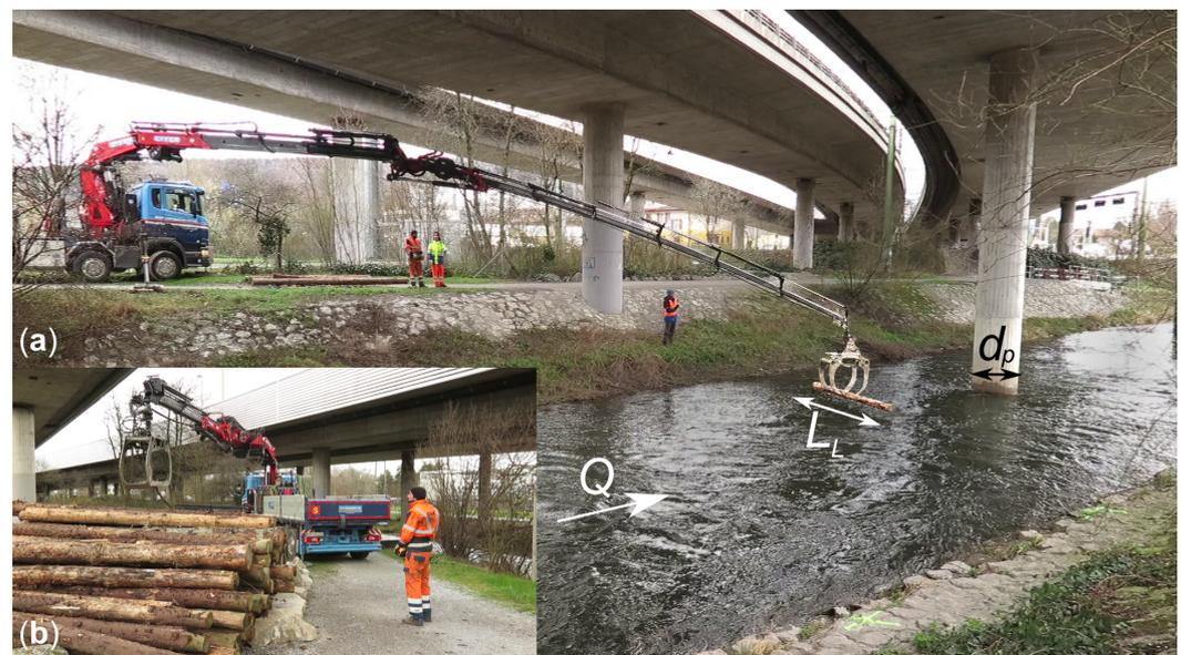
**Figure 2.** (a) Test site at the River Glatt with a log being placed upstream of the bridge pier by a truck crane with discharge  $Q$ , log length  $L_L$ , and pier diameter  $d_p$ , and (b) log storage prior to the log placement in the river.
