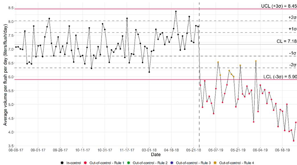
**Figure 8.** Shewhart Control Chart—Average volume per flush per day (female restrooms).
