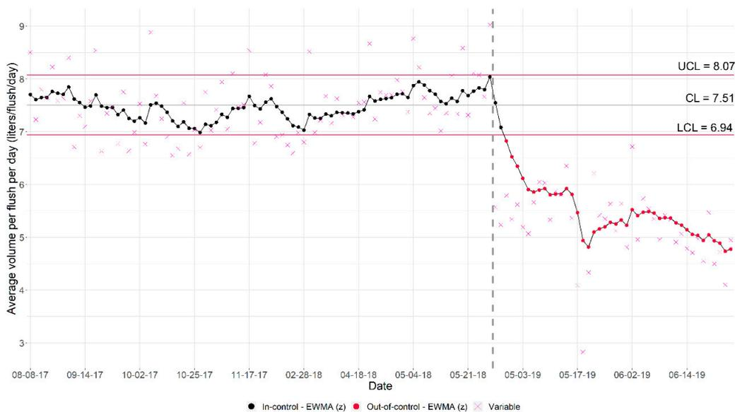
Figure 6. EWMA Control Chart—Average volume per flush per day.
