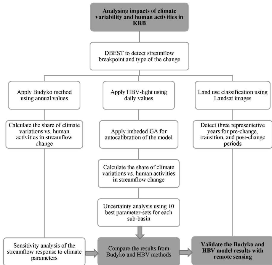
Figure 2. Flowchart of the implemented methodology.
