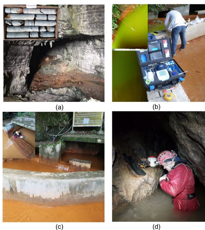
Figure 3. Investigation methods: (a) karst core sample from borehole YR-1; (b) water quality detection; (c) pollution in the Longdong Spring; (d) diving exploration in Sinkhole No.5.
