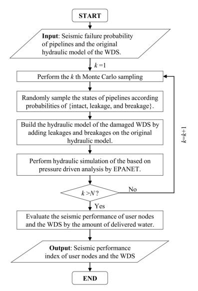
Figure 6. Flowchart of probabilistic seismic performance analysis of WDS based on MCS.
