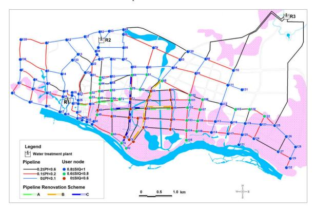
Figure 13. Seismic performance of the original WDS and the pipeline renovation schemes.
