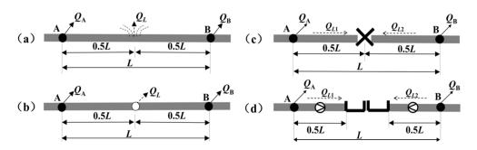
**Figure 5.** Diagram of pipeline damages and the hydraulic model of damages. (**a**) Diagram of leak. (**b**) Hydraulic mode of leak. (**c**) Diagram of break. (**d**) Hydraulic mode of break.
