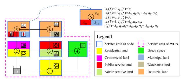
Figure 4. Land types in the service area of user nodes in the example WDS.
