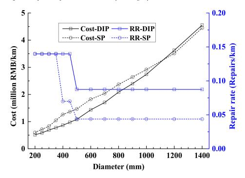
Figure 9. Construction cost and seismic repair rate of the pipelines in Z city.
