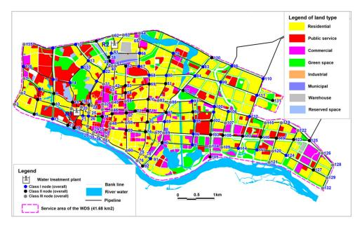
Figure 10. Land types in the service area of WDS in Z city and the overall importance of user nodes.
