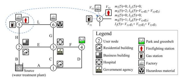
Figure 3. Layout of the example WDS and the service facilities of user nodes.
