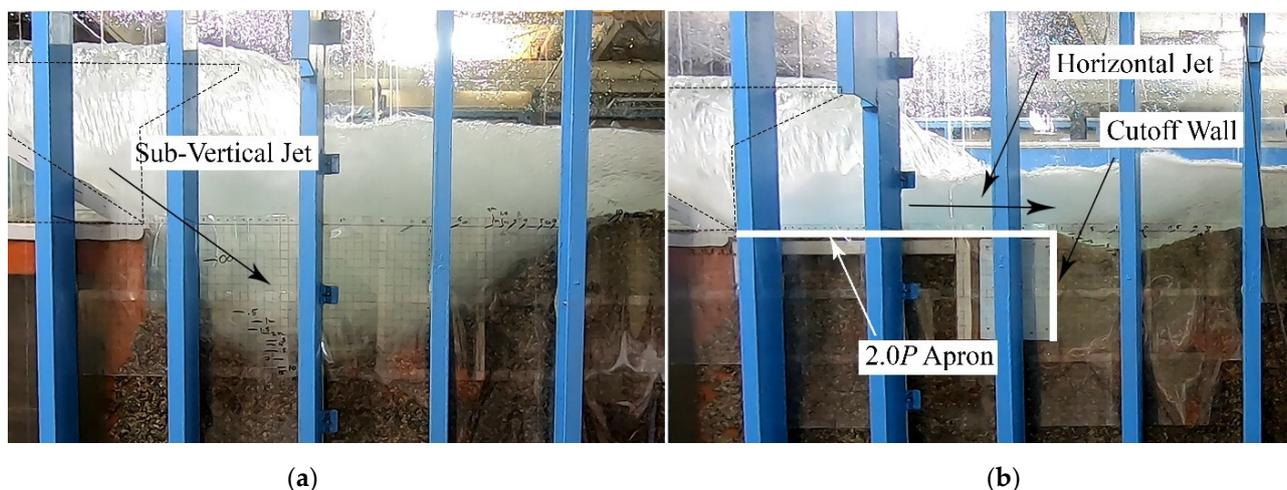
**Figure 3.** Photographs from experiments under identical hydraulic conditions: (a) Reference test (Run 14); (b) Scour protection via horizontal apron and cutoff wall (Run 23).
