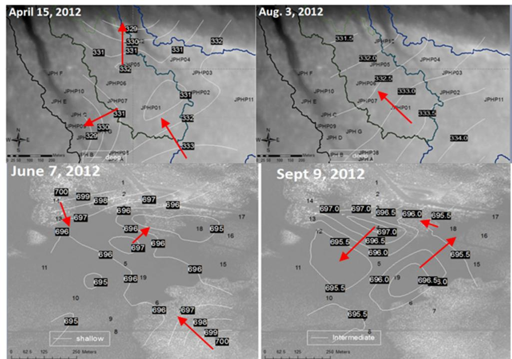
**Figure 3.** Maps showing hydraulic head elevations and inferred flow directions: for JPH (**top left**) April 2012, (**top right**) August 2012; and, for ML (**bottom left**) June 2012, and (**bottom right**) September 2012.
