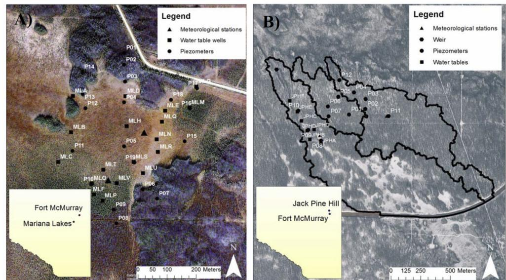
**Figure 2.** Location of instrumentation installed at (A) ML and (B) JPH. Note the scale differences in (A,B). Colours at ML depict uplands (purple), bogs (green), and fens (brown). Outlines at JPH depict delineated drainage areas including the rich fen (unit located to the southwest) and upland terrain units.
