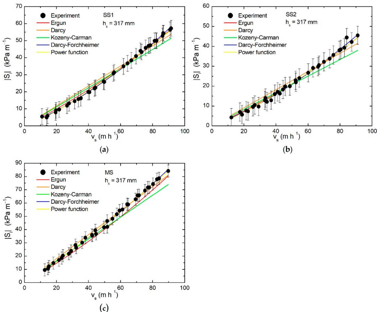
**Figure 2.** Regression fits of the absolute value of the observed momentum sink term in 200 mm of (a) silica sand 1, (b) silica sand 2, (c) microspheres as a function of the superficial velocity for Darcy Equation (7) (linear), Darcy-Forchheimer Equation (9) (quadratic) and power function Equation (11) (logarithmic). Trends from Kozeny-Carman Equation (8) and Ergun Equation (10) are also shown. Uniform flow in these 200 mm was assumed.
