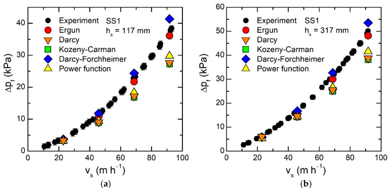
**Figure 5.** Filter pressure drop as a function of the superficial velocity experimentally observed and simulated using Equations (7)–(11) for the porous media (SS1) with sand height above the base plate equal to (a)  $h_s = 117 \text{ mm}$ ; (b)  $h_s = 317 \text{ mm}$ .
