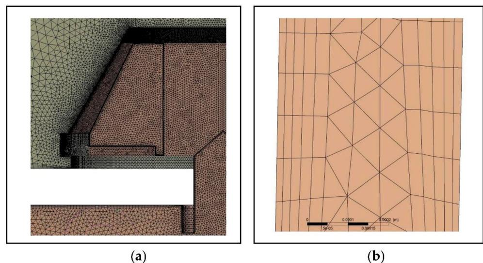
**Figure 3.** Detail of the mesh applied to (a) the influence zone of the underdrain element (half section view); (b) the open area of the slots of the underdrain (see layers of 5 prisms attached to lateral walls; the total length of the yardstick is 0.2 mm).
