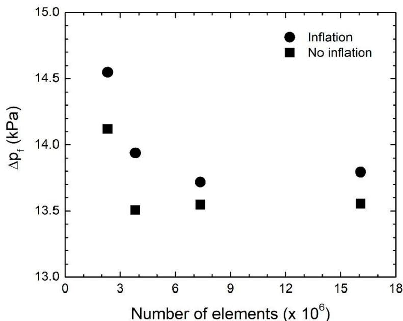
**Figure 4.** Filter pressure drop simulated with Ergun equation using grids of different element size with and without inflation layers. SS2 granular media and volumetric flow equal to  $0.4 \text{ L s}^{-1}$ .
