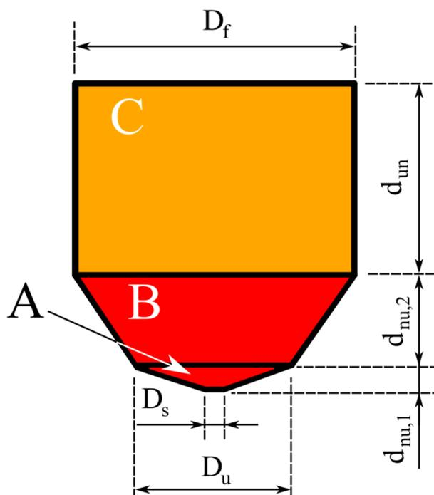
**Figure 12.** Schematic view of the three regions defined to calculate the pressure drop in the granular bed. Flow is non-uniform in zones A and B (red) and uniform in zone C (orange). See text for definitions of the parameters.
