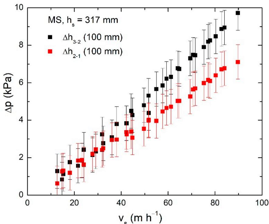
**Figure 14.** Experimental data of pressure drop in the granular bed at slab located between  $h_3 = 300$  mm and  $h_2 = 200$  mm ( $\Delta h_{3-2}$ ) and at slab located between  $h_2 = 200$  mm and  $h_1 = 100$  mm ( $\Delta h_{2-1}$ ). Microspheres (MS) case with  $h_s = 317$  mm.
