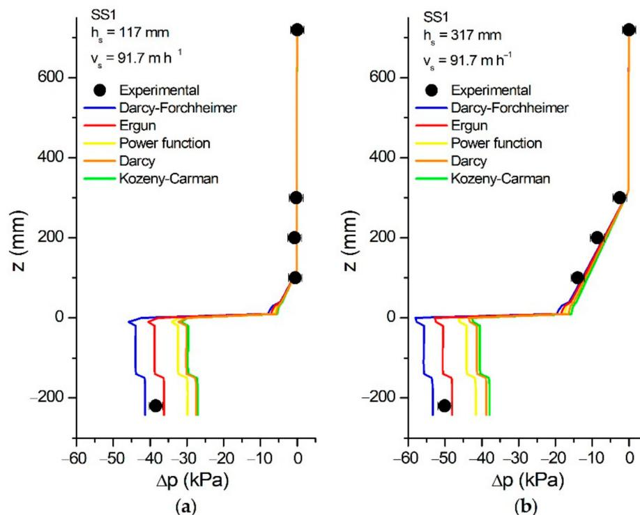
**Figure 9.** Differences between horizontally averaged values of pressure at different heights and pressure inlet for case (a)  $h_s = 117$  mm and (b)  $h_s = 317$  mm both at  $Q = 0.81 \text{ s}^{-1}$  and SS1 media.
