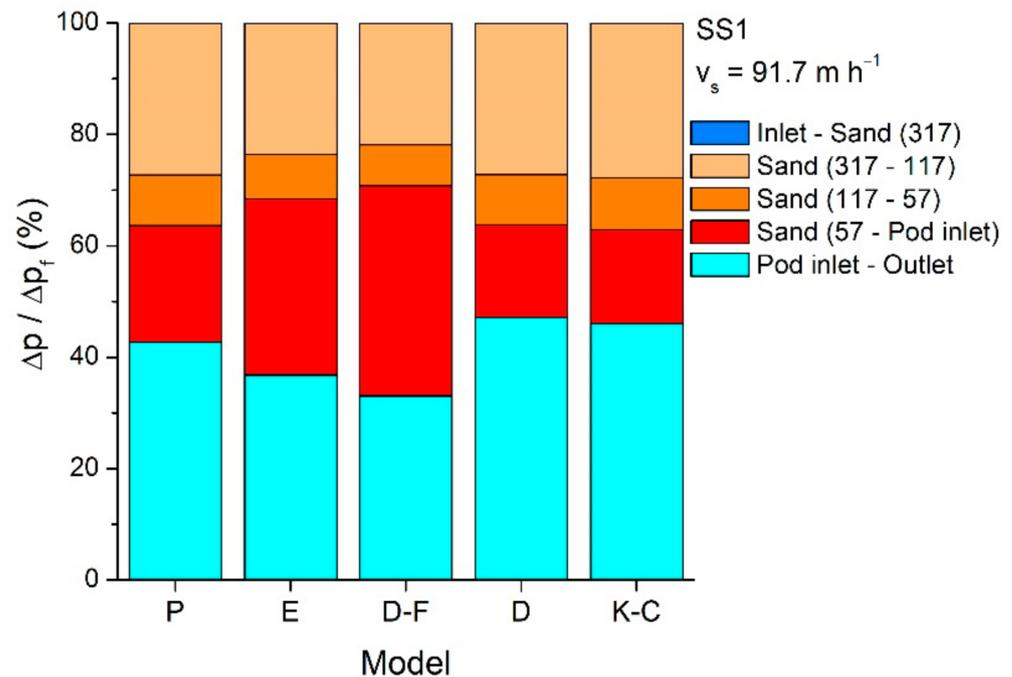
**Figure 8.** Pressure drop  $\Delta p$  at different filter regions normalized to the total filter pressure drop  $\Delta p_f$  for case  $h_s = 317$  mm,  $Q = 0.8$  L s<sup>-1</sup> and SS1 media using different porous media momentum sink equations. P = Power function, E = Ergun, D-F = Darcy-Forchheimer, D = Darcy, K-C = Kozeny-Carman. Numbers in parentheses refer to the vertical height  $z$  above the underdrain base plate in mm.
