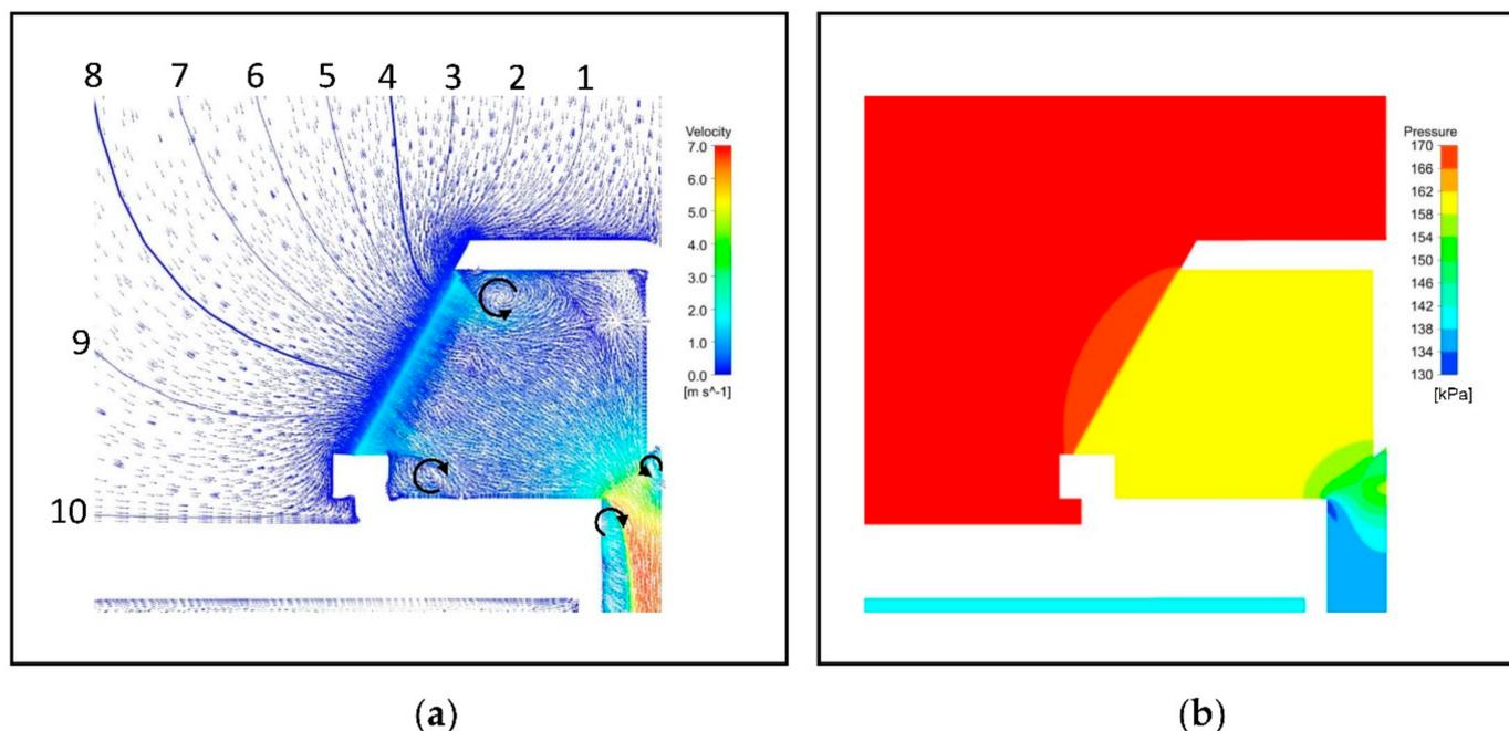
**Figure 11.** (a) Velocity vectors and (b) pressure contours at the underdrain region for case SS1 with Ergun model,  $Q = 0.8 \text{ L s}^{-1}$ ,  $h_s = 317 \text{ mm}$  in a vertical plane at  $44^\circ$  angular position from the symmetry plane (crosses through the middle of a slot).
