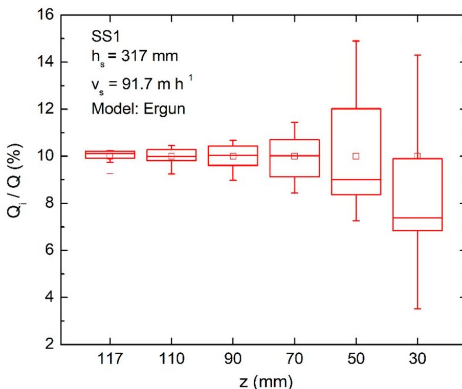
**Figure 10.** Box-plot of normalized volumetric flow rates through 10 horizontal annular plus circular centered sectors at different heights above the base plate. Case  $h_s = 317$  mm at  $Q = 0.8$  L s<sup>-1</sup> and SS1 media with Ergun equation.
