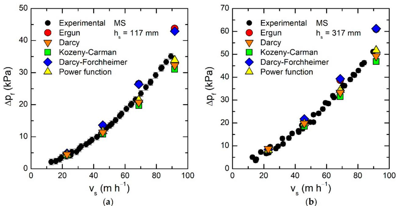
**Figure 7.** Filter pressure drop as a function of the superficial velocity experimentally observed and simulated using Equations (7)–(11) for the porous media (MS) with micro spheres height above the base plate equal to (a)  $h_s = 117$  mm; (b)  $h_s = 317$  mm.
