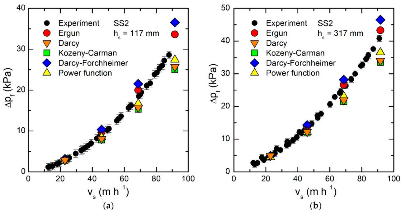
**Figure 6.** Filter pressure drop as a function of the superficial velocity experimentally observed and simulated using Equations (7)–(11) for the porous media (SS2) with sand height above the base plate equal to (a)  $h_s = 117 \text{ mm}$ ; (b)  $h_s = 317 \text{ mm}$ .
