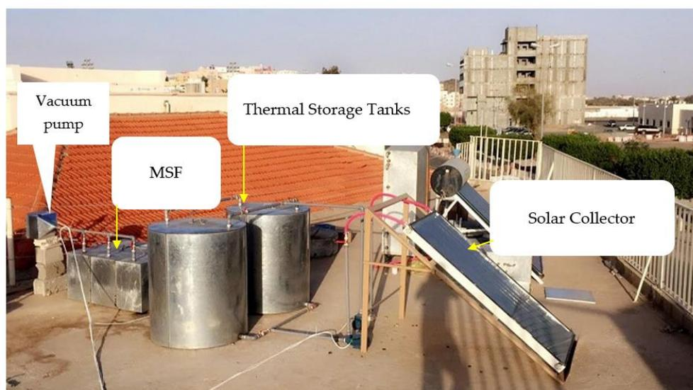
**Figure 2.** A photograph of the experimental system.
